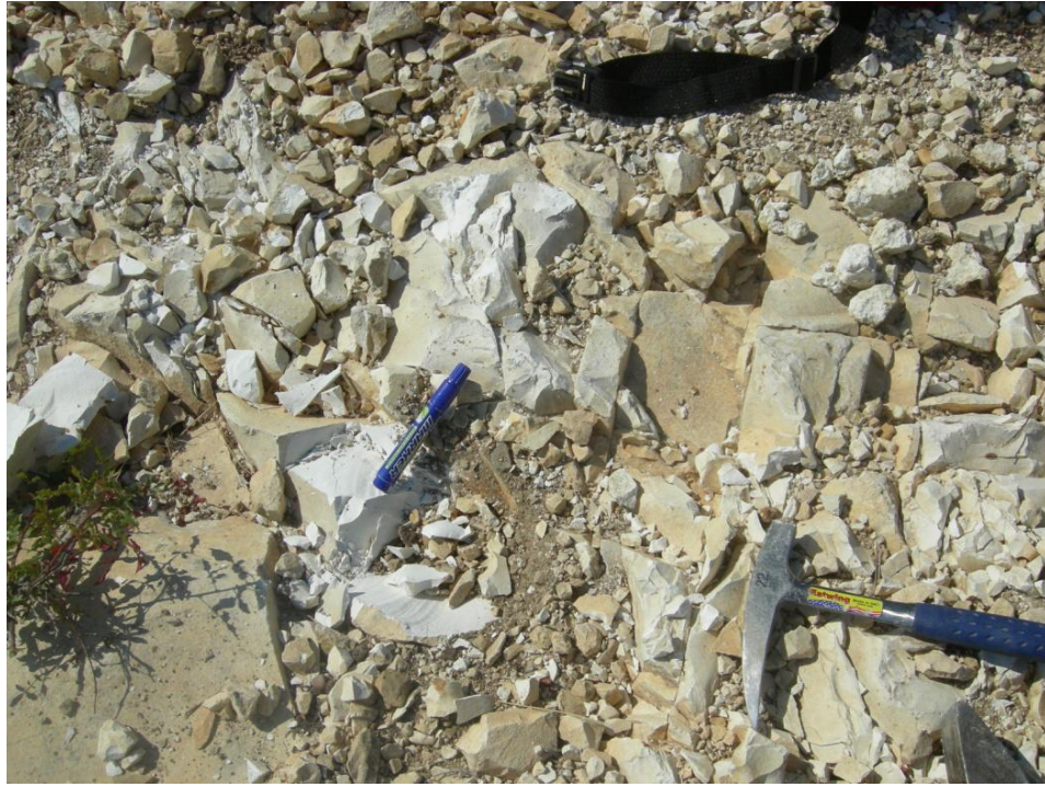
Figure 3.5 A view from Foça Tuff, which is soft, homogeneous and white in color.
