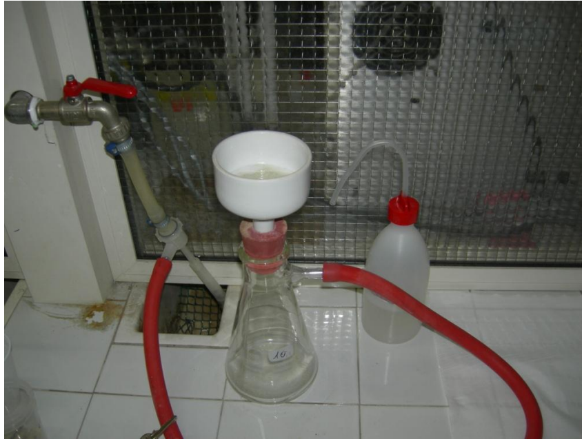
Figure 4.4 Vacuum filtration setup of hardened paste after washing with acetone.
