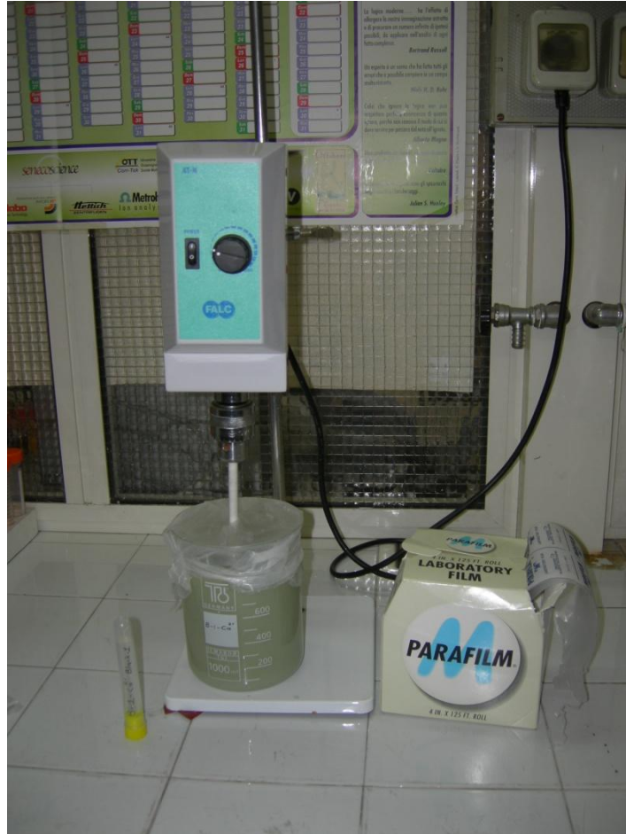
Figure 4.3 Experimental set-up for cross exchange method (CEM).
