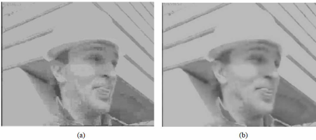
Figure 2.9: Deblocking filter effect a) Without deblocking filter b) With in-loop deblocking filter [54]
