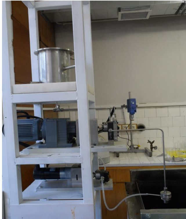
Figure 3.4. Hollow fiber spinning system with polymer dope and bore liquid pumps
