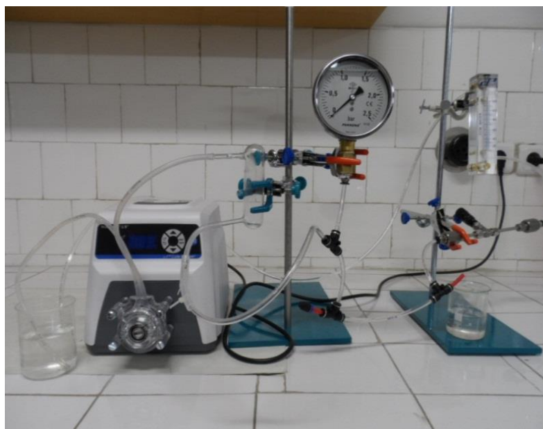
Figure 3.8. Retention test set up picture of hollow fiber membranes
