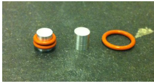
Figure 3.6 Specimen and silicone O-ring configuration to attach the thermocouple to the specimen
