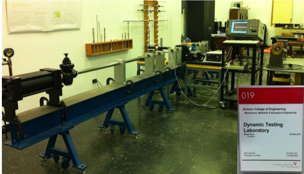
Figure 3.7 A view of SHPB at Dynamic Testing Laboratory of IIT
