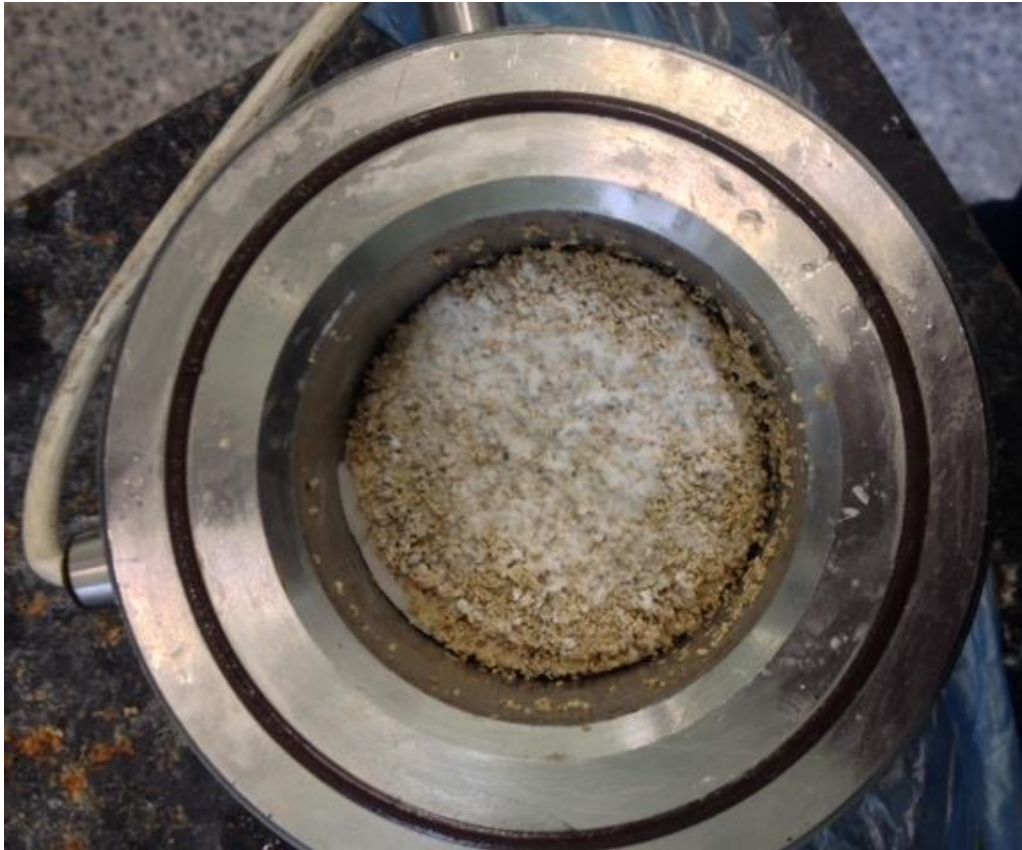
Figure 6-9: Clear picture of formed hydrate in sand sediments
