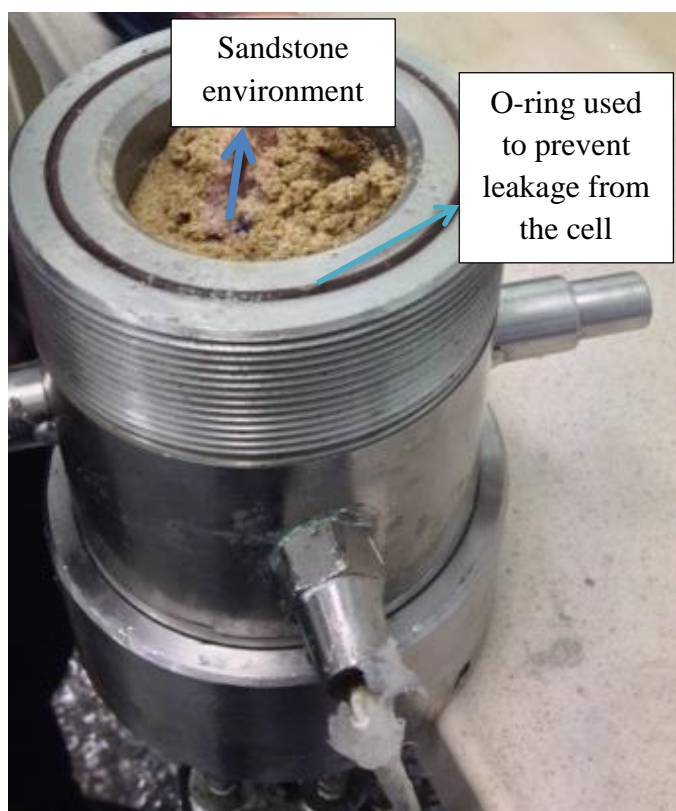
Figure 5-1: High pressure cell used in experiments
