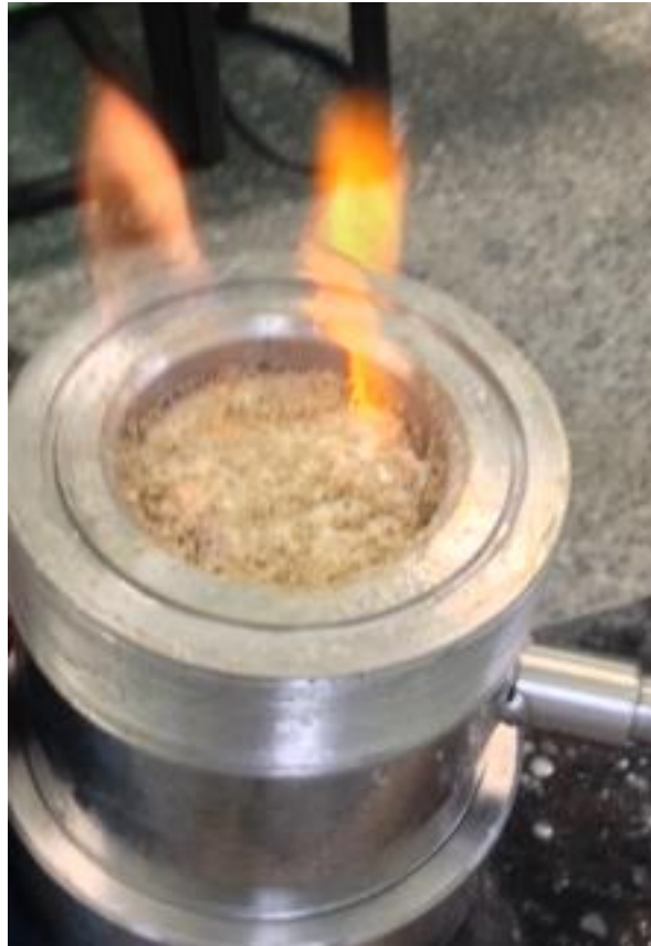
Figure 6-10: Inflammation of hydrate formed in sand sediments
