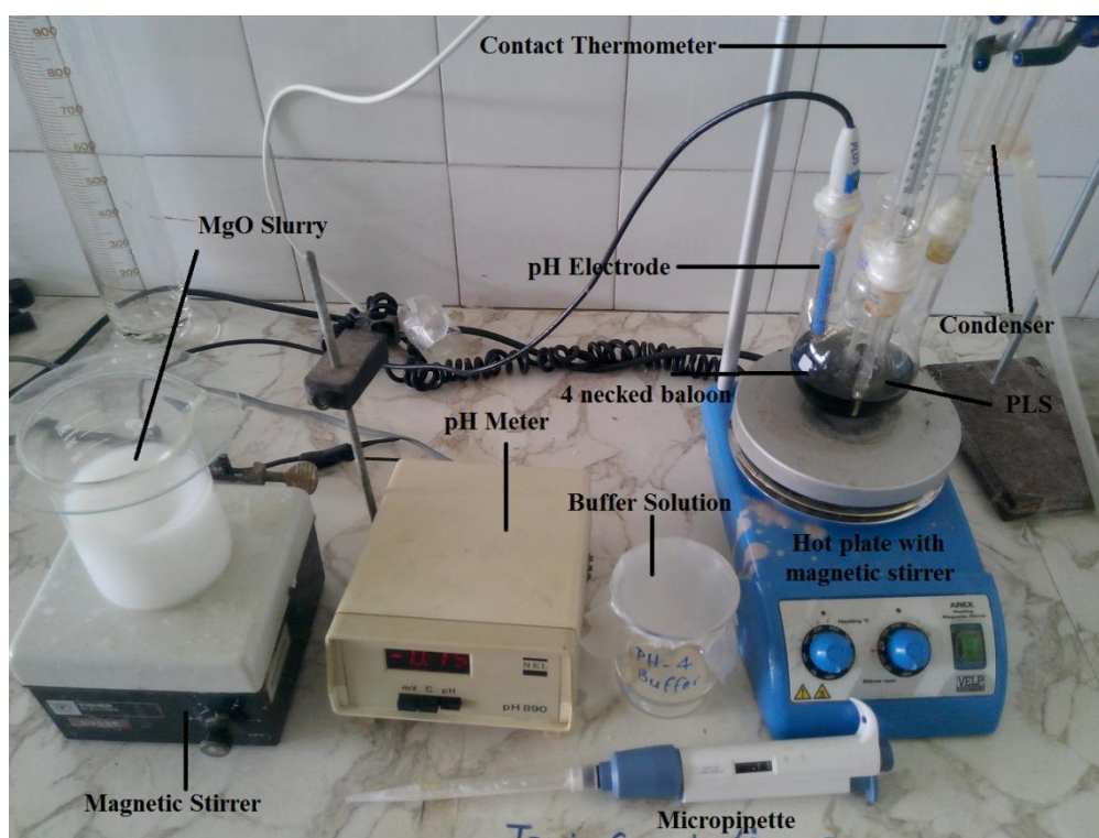
Figure 26: Experimental set-up for neutralization and iron removal
