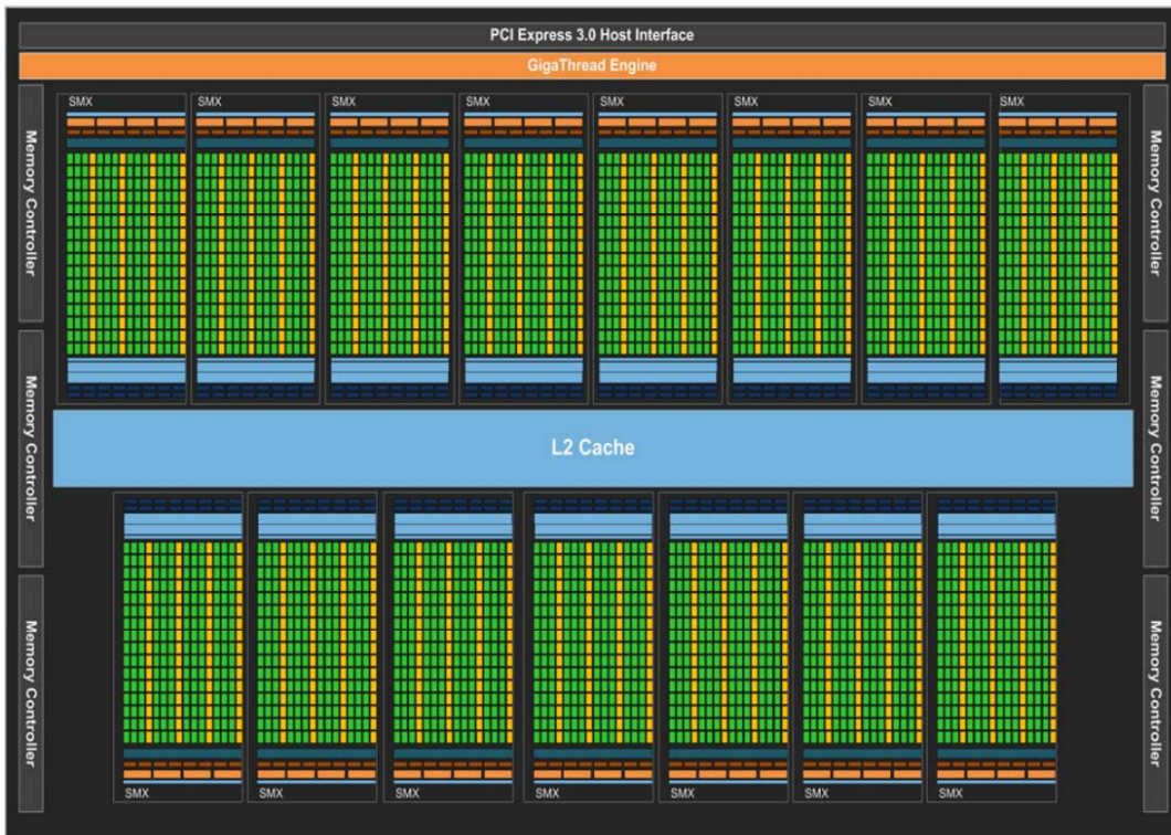
Figure 2.9: Nvidia Kepler Architecture. Adapted from "NVIDIA Kepler GK110 Architecture Whitepaper", by Nvidia Corporation, 2012, p. 6. Copyright 2012 by Nvidia Corporation [11]
