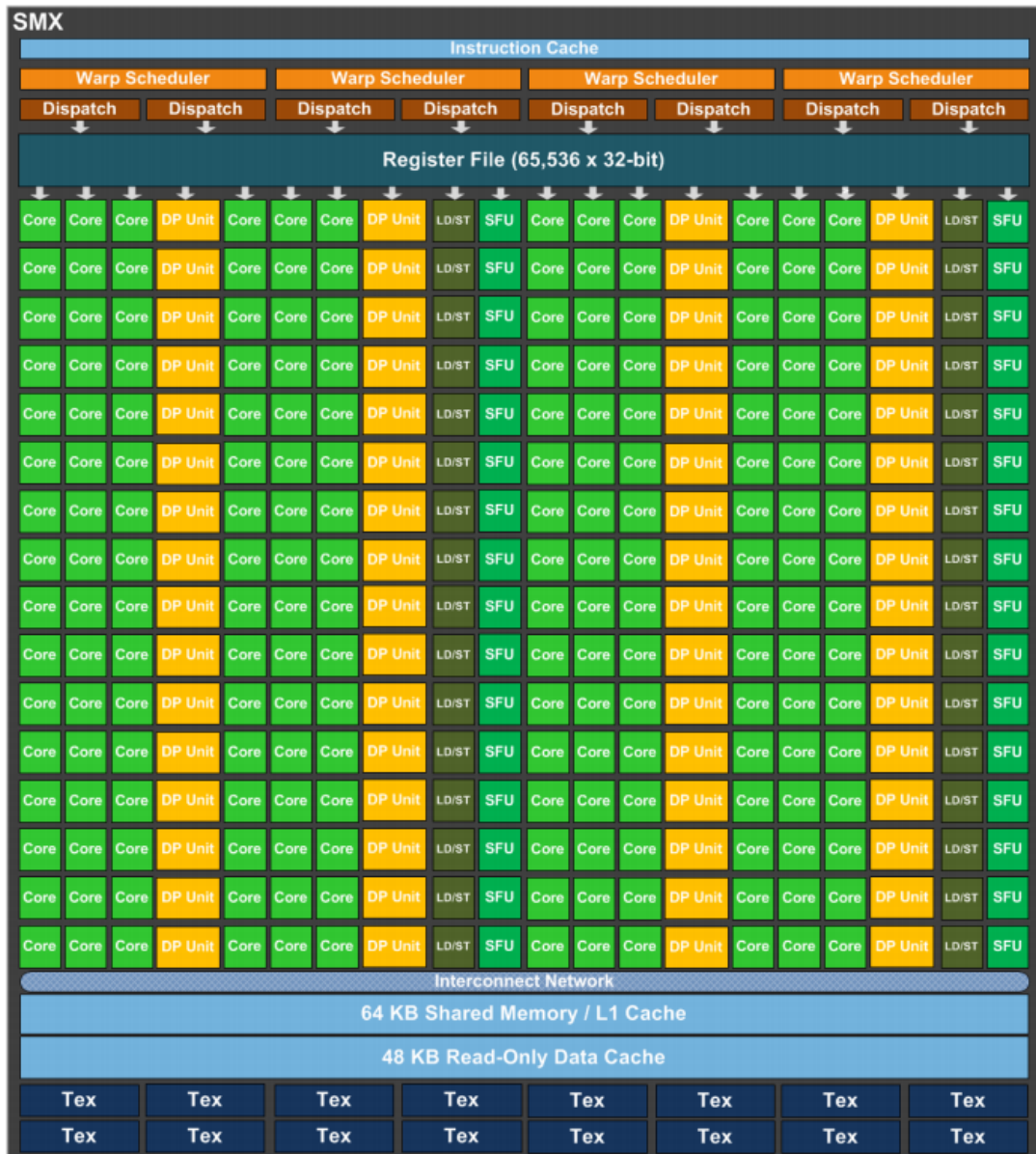
Figure 2.10: Nvidia Kepler Streaming Multiprocessor Architecture. Adapted from "NVIDIA Kepler GK110 Architecture Whitepaper", by Nvidia Corporation, 2012, p. 8. Copyright 2012 by Nvidia Corporation [11]
