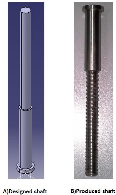
Figure2.9. The Designed (A) and Produced (B) Shaft
