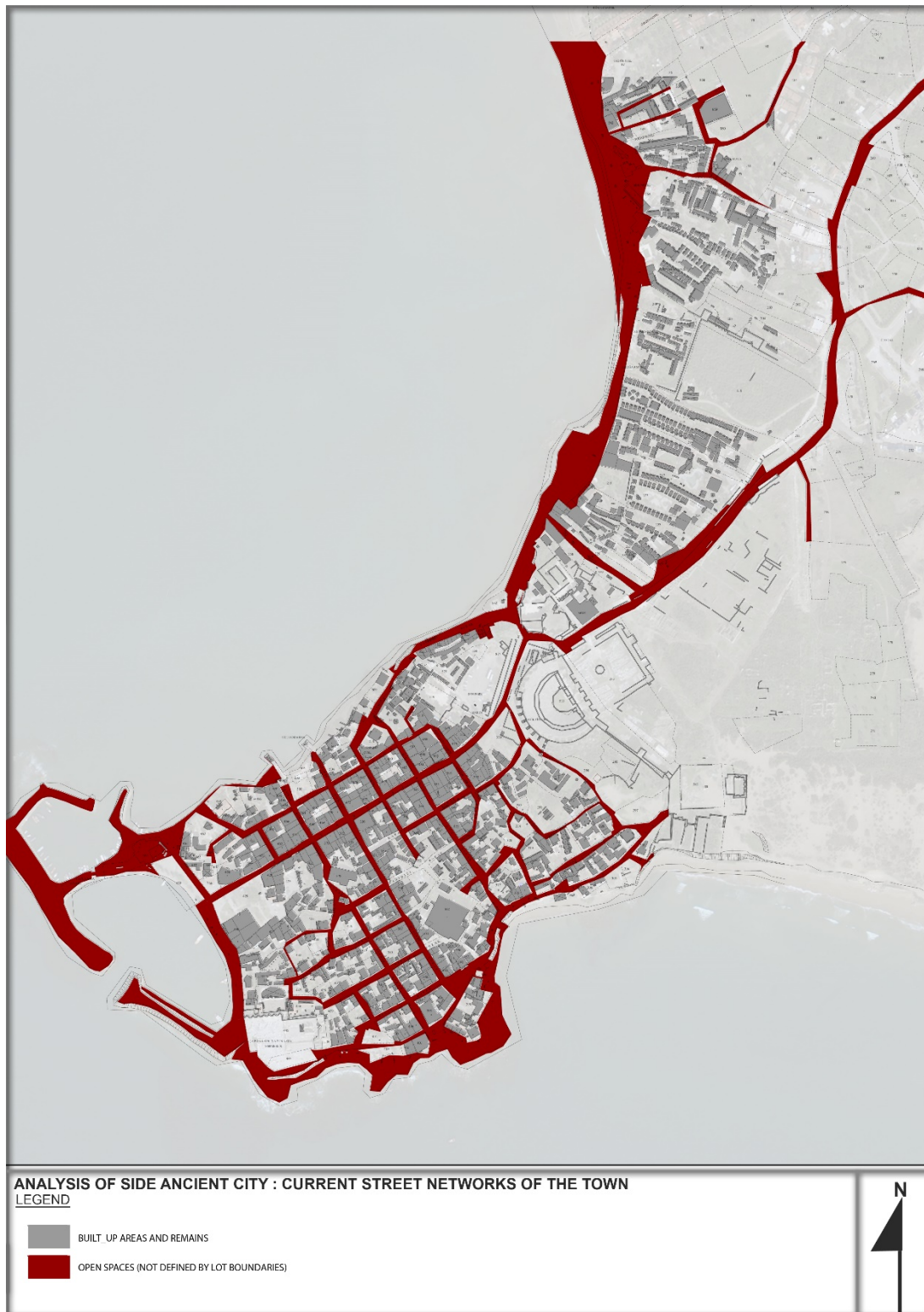
Figure 2. 46: The analysis of the current street networks in the town (prepared by the author)
