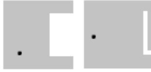
Figure 2.6 Notch loaded multi frequency patch antennas
