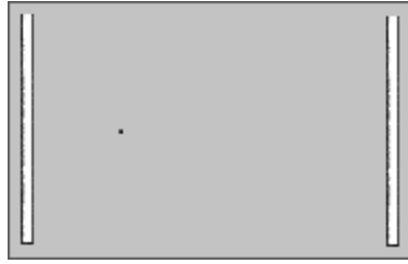
Figure 2.8 Dual band slot loaded patch antenna
