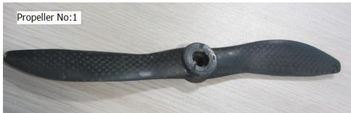
Figure 4.2 Prototype of Turbotek Prop6 (10x7) Propeller [24]
