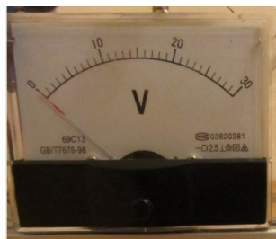
Figure A.7 Analog DC Voltmeter 30V
