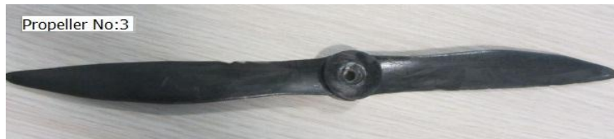
Figure 4.10 Prototype of Turbotek eProp2 (12x7) Propeller [26]
