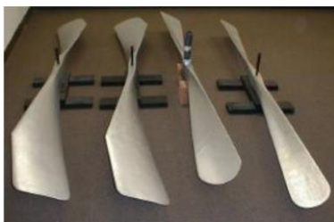
Figure 1.3 Reproduction of Wright Brothers' propeller [4]
