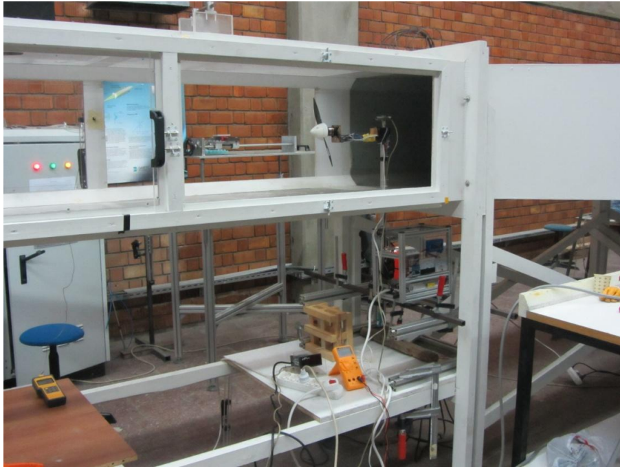
Figure 3.16 General view of the installation of the propeller test apparatus to the test section of the wind tunnel
