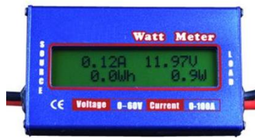
Figure A.6 Digital power meter
