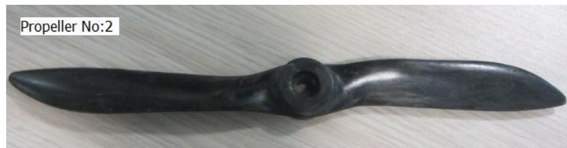
Figure 4.6 Prototype of Turbotek Prop1 (10x6) Production Propeller [25]
