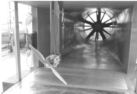
Figure 1.20 Wind tunnel with the experimental rig installed
