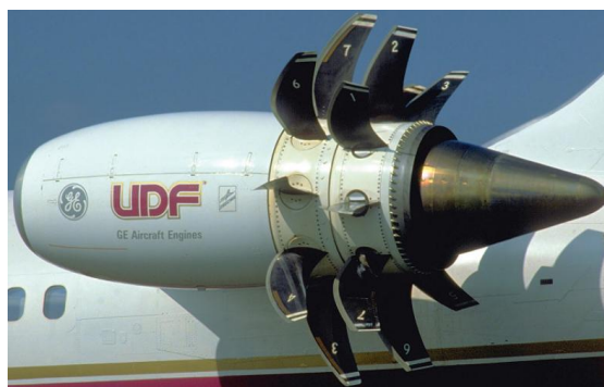
Figure 1.6 General Electric GE-36 Unducted Fan (UDF) with two eight-bladed sets of contra-rotating blades [6]
