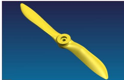
Figure 4.5 3D CAD model of Turbotek Prop1 (10x6) Propeller [25]
