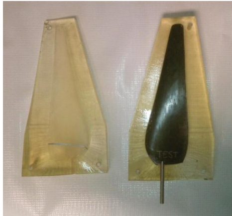
Figure 1.9 Propeller blade molds with test lay-up
