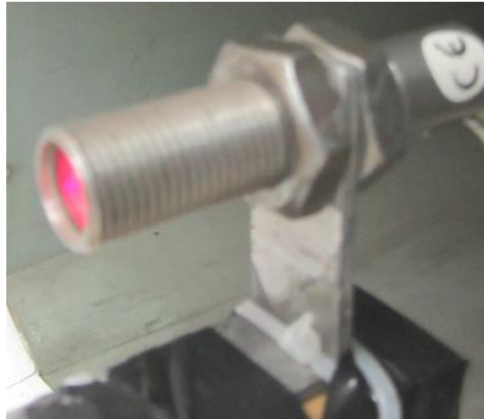
Figure 3.9 Laser sensor of the tachometer
