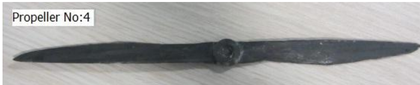
Figure 4.14 Prototype of Turbotek eProp1 (10x7) Propeller [27]
