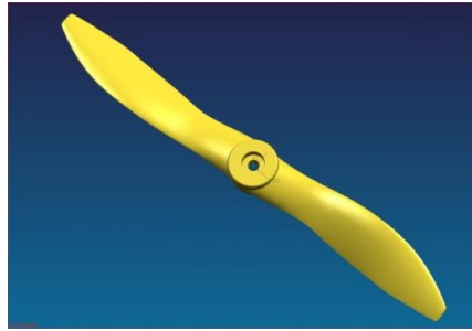
Figure 4.1 3D CAD model of Turbotek Prop6 (10x7) Propeller [24]
