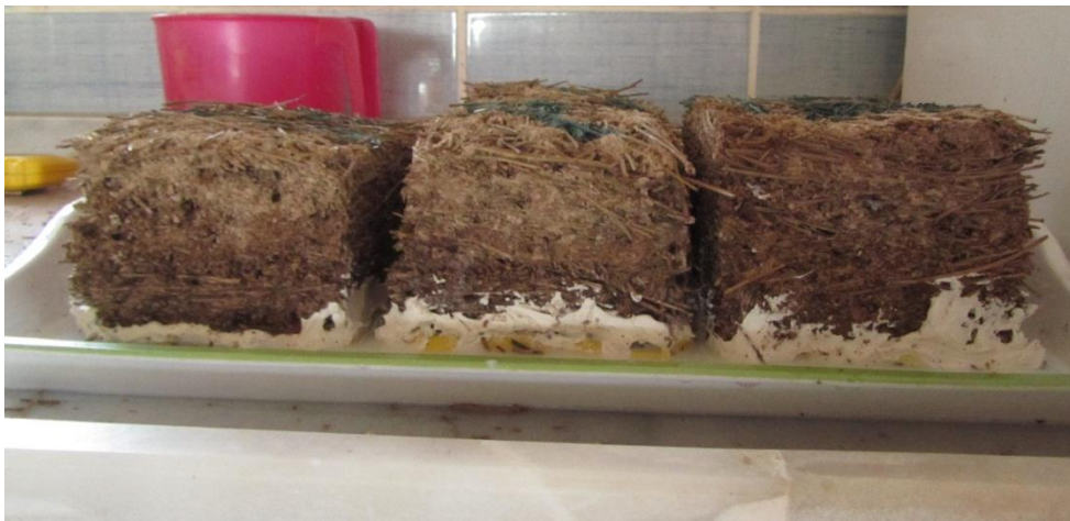
Figure 56: Samples are shown being laid on water.
