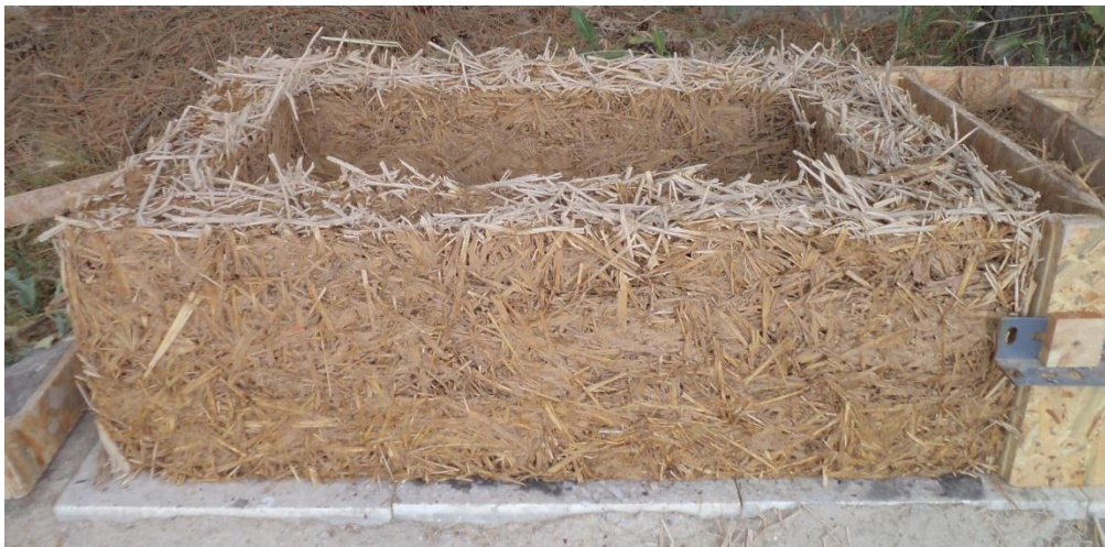
Figure 53: Pine-needle LWL box directly after being taken out of the mold.
