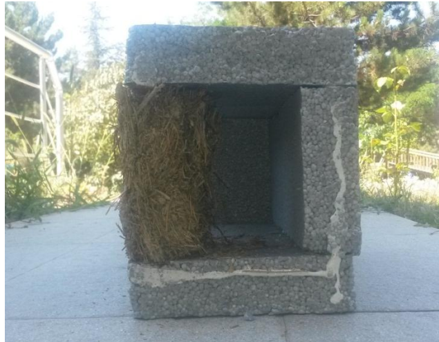
Figure 58: Vapor resistivity test box made of 5 cm thick polystyrene is seen with one of the pine-needle LWL sample. The box is not closed and sealed yet.
