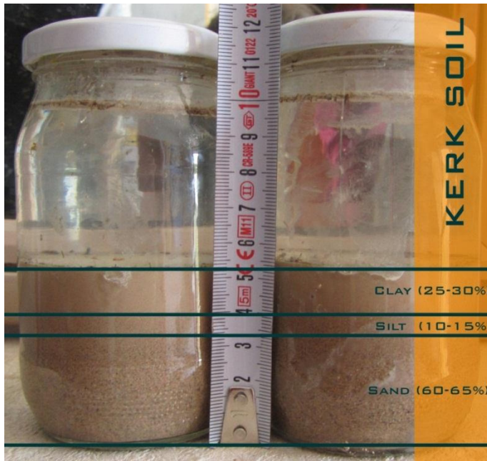
Figure 63: Result of bottle test for KERK Soil.
