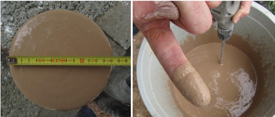
Figure 47: On the left: slip loam puddle has around 14 cm diameter viscosity. On the right: Viscosity test according to the trace of slip loam on the skin.
