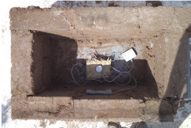
Figure 117: Mud brick box open with data logger and surface sensor inside.
