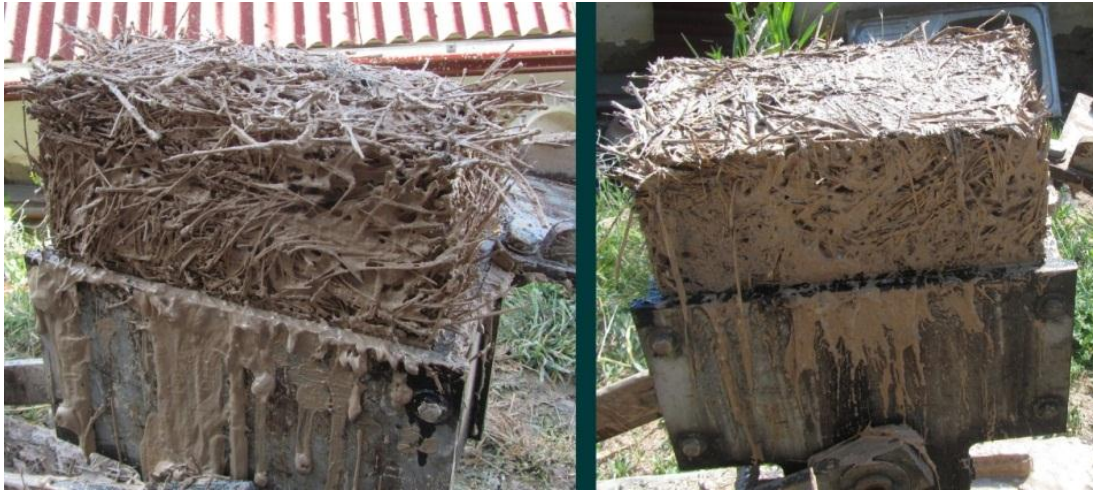
Figure 65: Pressed Blocks prepared with respectively LPN (left) and straw (right).
