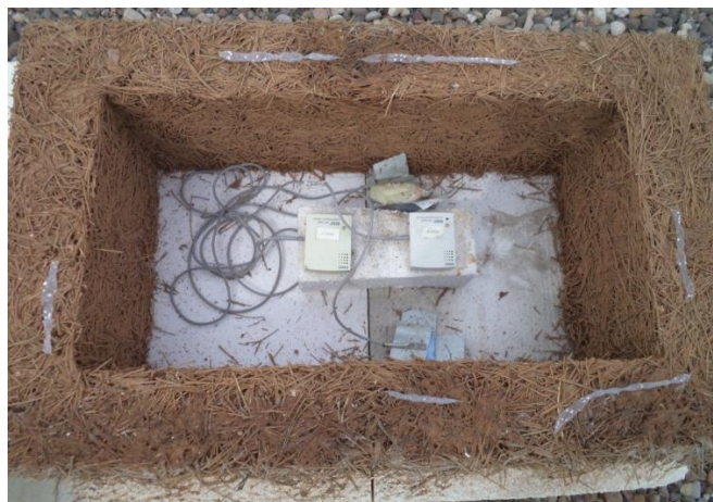
Figure 119: LPN-METU-1 box open with data logger and surface sensor inside.
