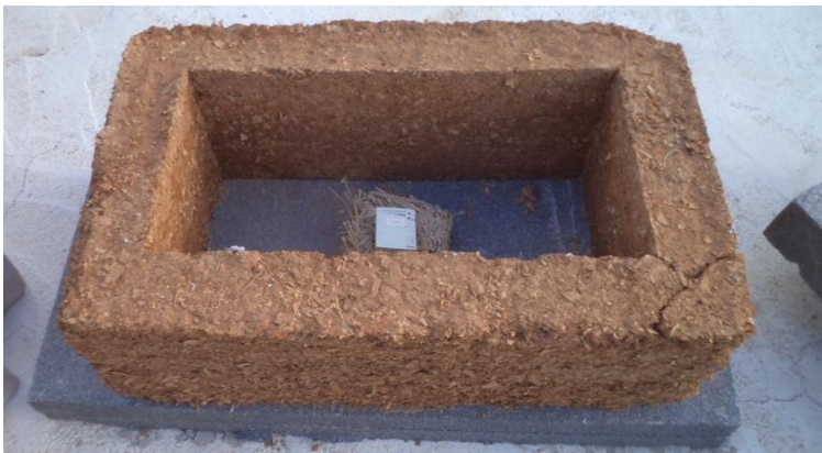
Figure 115: Woodchips LWL box open with data logger inside.
