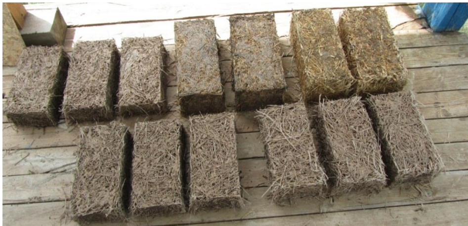
Figure 51: Brick samples made of both pine needles and straw.
