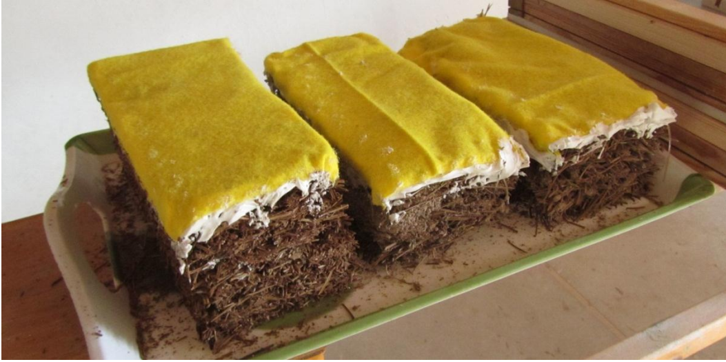
Figure 55: Samples covered with cloth and sealed with silicon.
