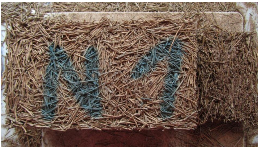
Figure 54: The difference of trimmed and non-trimmed side of brick sample is seen.
