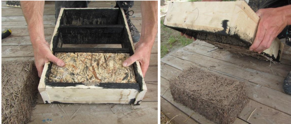
Figure 50: Brick samples are taken out of molds after 12 hours to avoid expansion.
