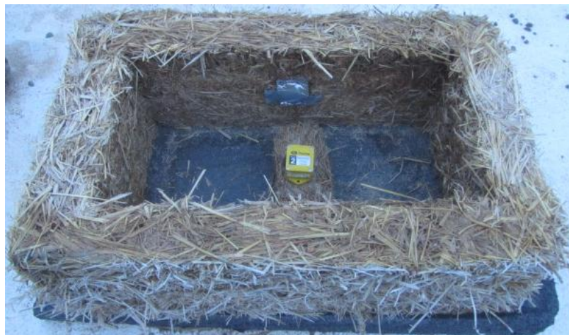
Figure 113: STRAW-KERK-2 box open with data logger and surface sensor inside.
