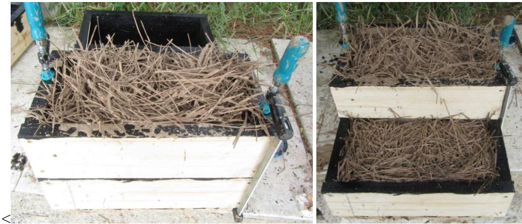
Figure 49: Two volume of mix is tamped into one volume of mold to be able to obtain a condensed brick sample.
