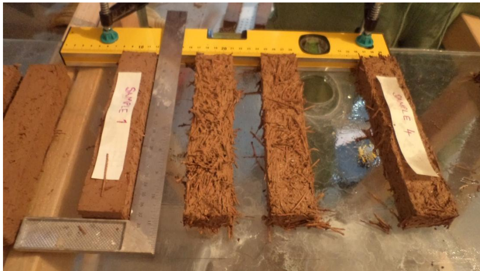
Figure 44: Some of the samples are shown on the oiled glass. The samples were aligned by meter.
