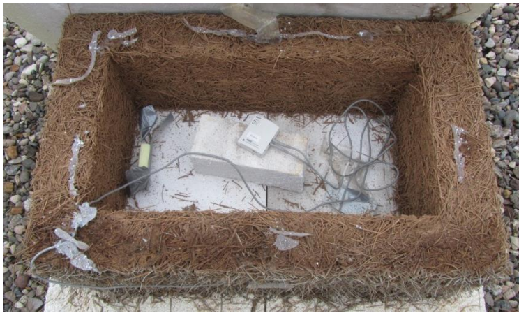
Figure 121: LPN-METU-2 box open with data logger and surface sensor inside.
