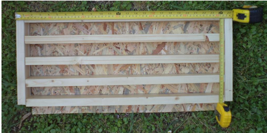
Figure 37: Shrinkage box that is used for Linear Shrinkage Test.
