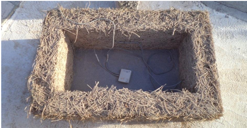
Figure 109: LPN-KERK-3 box open with data logger inside.
