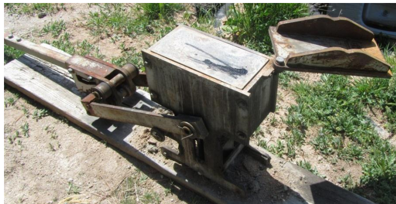
Figure 38: Pressed block machine in Kerkenes Eco Center.
