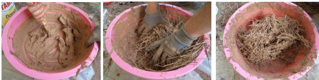
Figure 43: Preparation process of the mix for preliminary tests.
