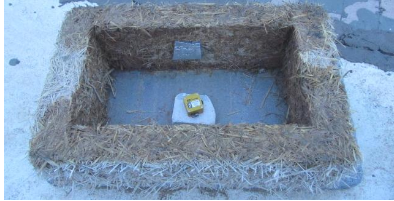
Figure 111: STRAW-KERK-1 box open with data logger and surface sensor inside.
