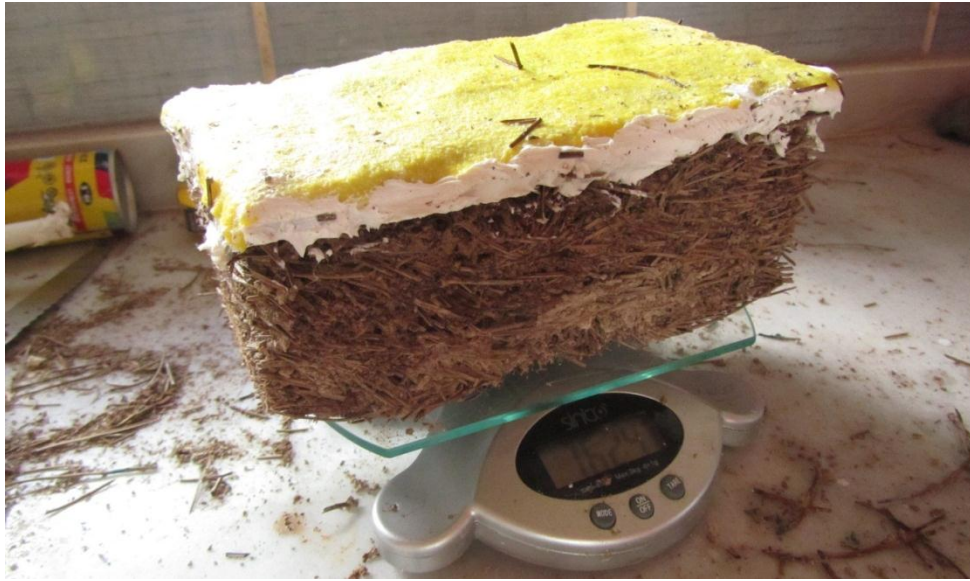
Figure 57: Sample is weighted after 1, 5, 14, 30 and 55 minutes.
