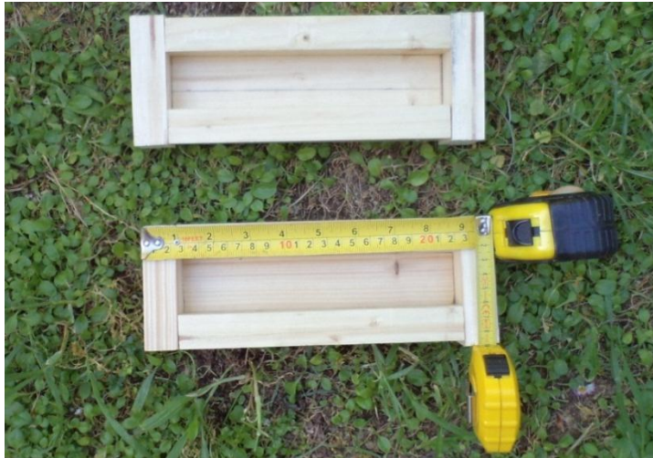
Figure 36: Shrinkage box according to TS-2514.
