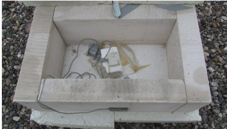
Figure 124: AAC box open with data logger and exterior surface sensor.
