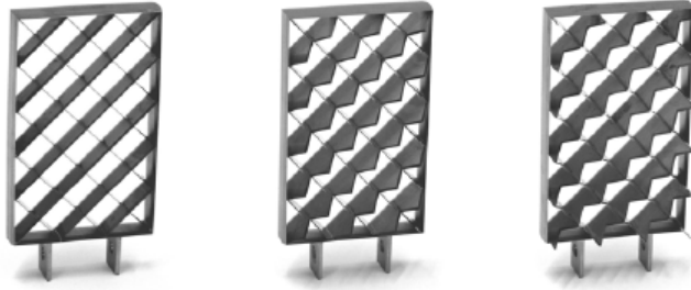
Figure 1.12: Flat (left), valley-type (center) and peak-type (right) grid fin models [30]
