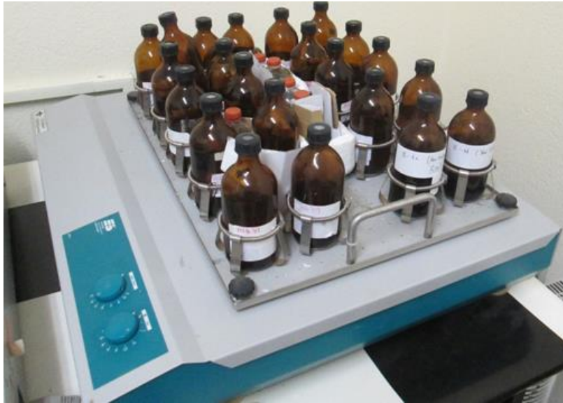
Figure 4.3 Setup of Set-B, incubated at the hot room ( 35\pm 2 °C) on a shaker (at 125 rpm)
