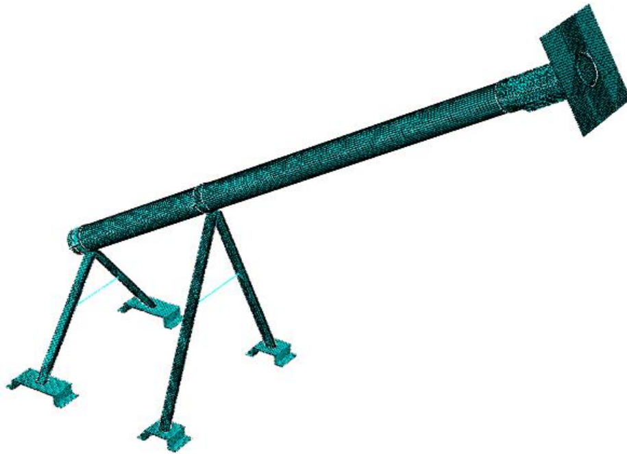
Figure 3-5: General mesh structure of the physical structure
