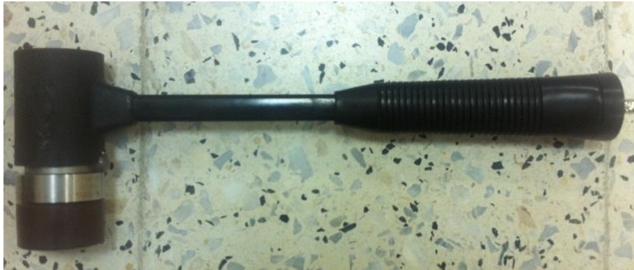
Figure 3-12: Impact hammer used in the modal tests
