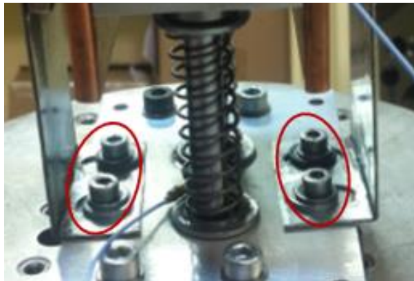
Figure 4-22: Slotted configuration of the magnet plates
