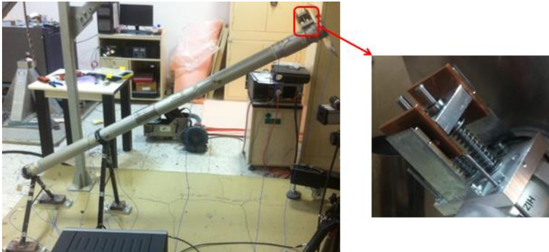
Figure 5-1: TVA location on the physical structure
