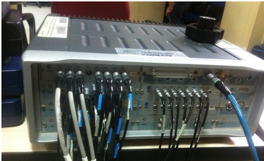
Figure 3-15: LMS hardware used in the modal tests
