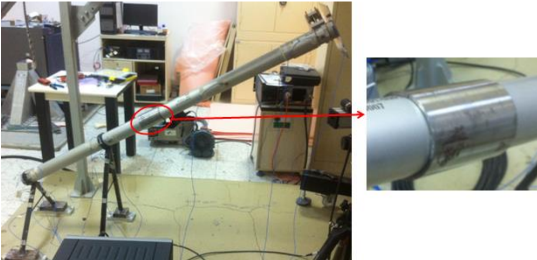
Figure 5-9: Attachment of the additional mass on the physical structure
