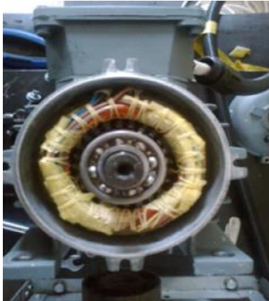
(a) Rotor ve stator
