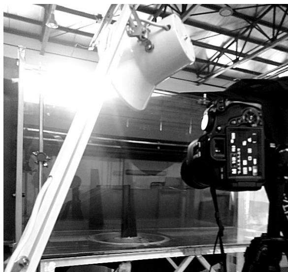
Figure 3.19 Oil Visualization Set-Up
