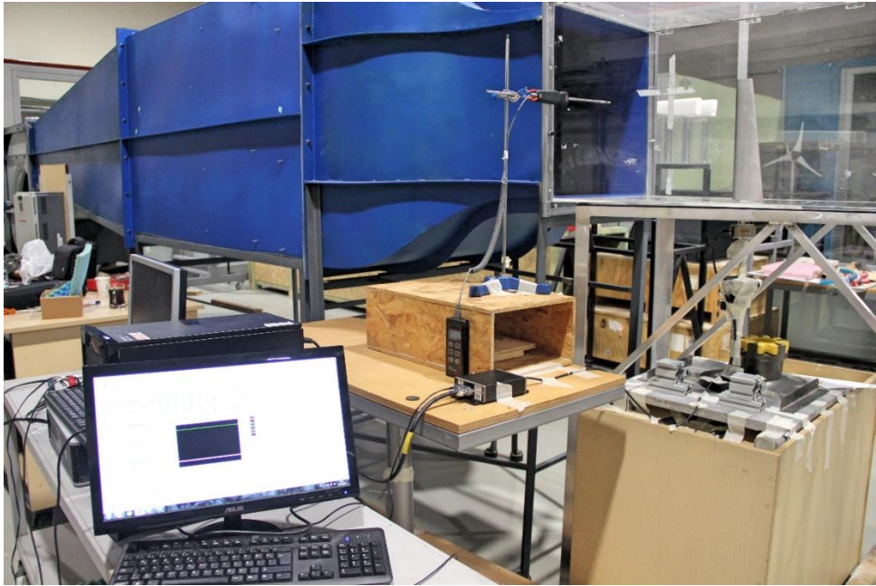
Figure 3.10 Load cell measurements set-up
