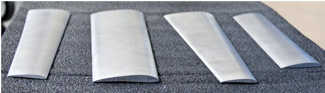
Figure 2.17 Manufactured wings side view from the tip chord (from left to right: Base Wing, Optimized Wing at 14 m/s, Morphed Wing at 10 m/s, Morphed Wing at 16.5 m/s)
