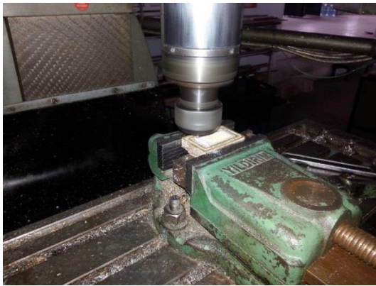
Figure 7.3- The milling machine used for creating the voids.
