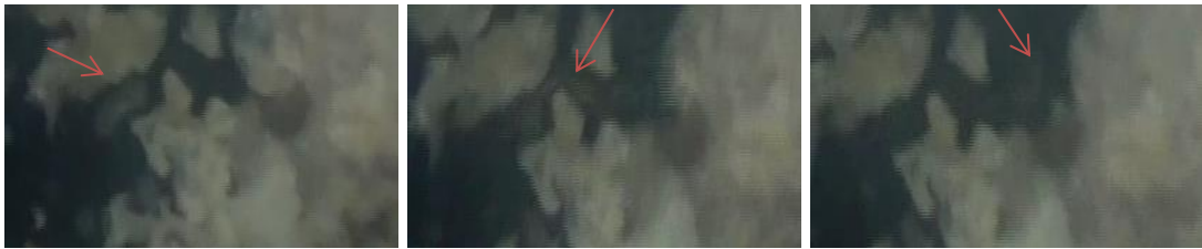
Figure 7.10- Jump process. Oil displaces water.
