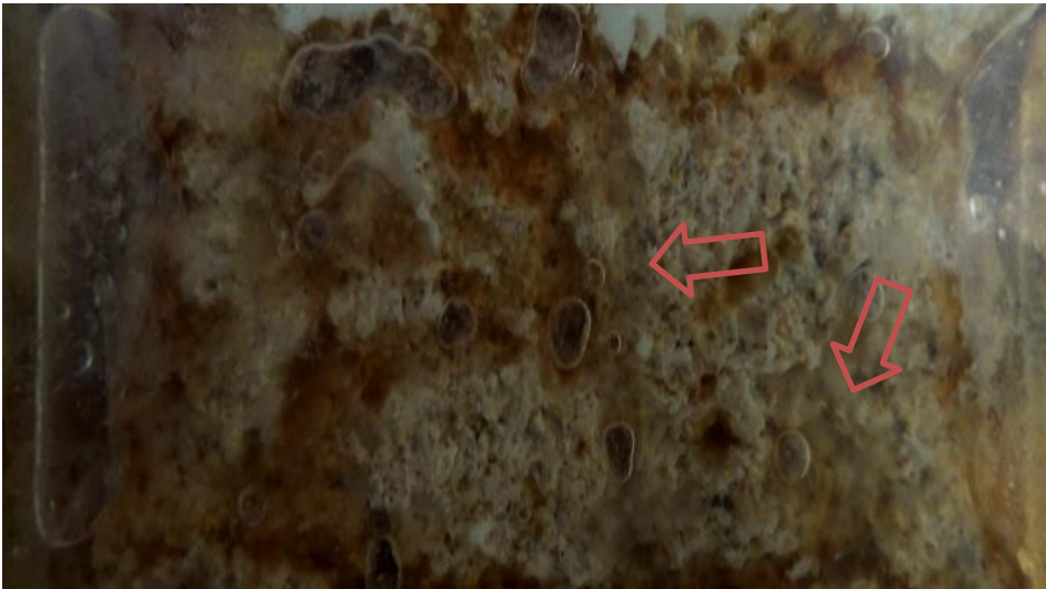
Figure 7.30- Top view after 90 minutes of injection of distilled water at a rate of 0.05 ml/min.
