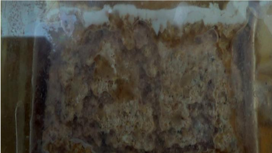
Figure 7.37- Top view after 3 hours of injection of liquid detergent solution at a rate of 0.05 ml/min.
