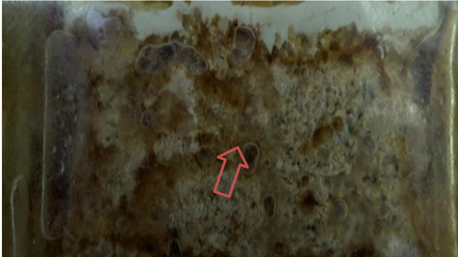
Figure 7.31- Top view after 3 hours of injection of distilled water at a rate of 0.05 ml/min.
