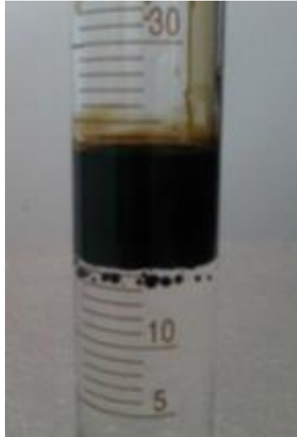
Figure 6.14- Oil particles suspended beneath the oil/brine interface.
