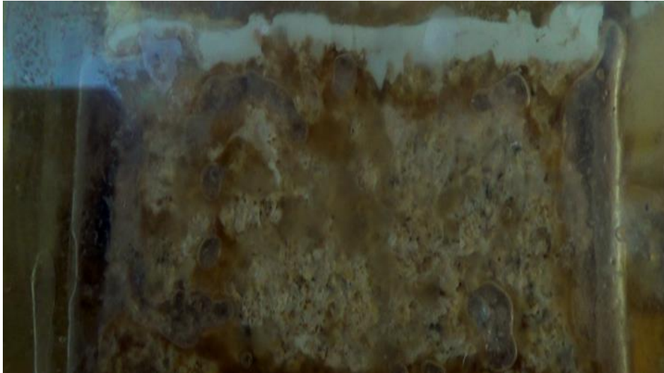
Figure 7.35- Top view after 60 minutes of injection of liquid detergent solution at a rate of 0.05 ml/min.
