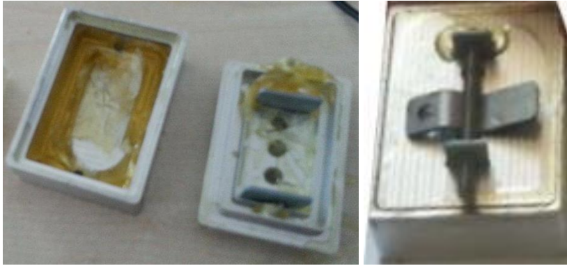
Figure 7.2- The mold into which the rock slice was inserted.
