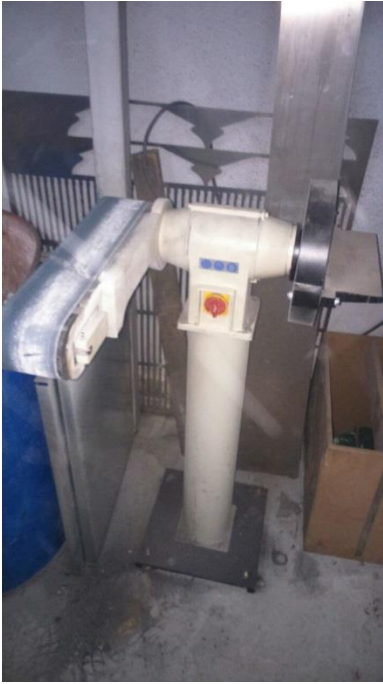
Figure 7.4- The band emery machine used for smoothing the surface of the rock slice.
