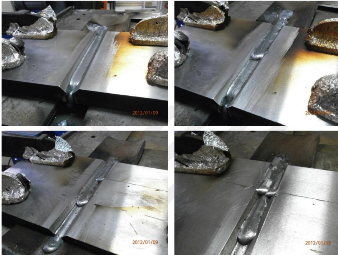
Figure 4.3 Welding of 2-pass and 4-pass configurations
