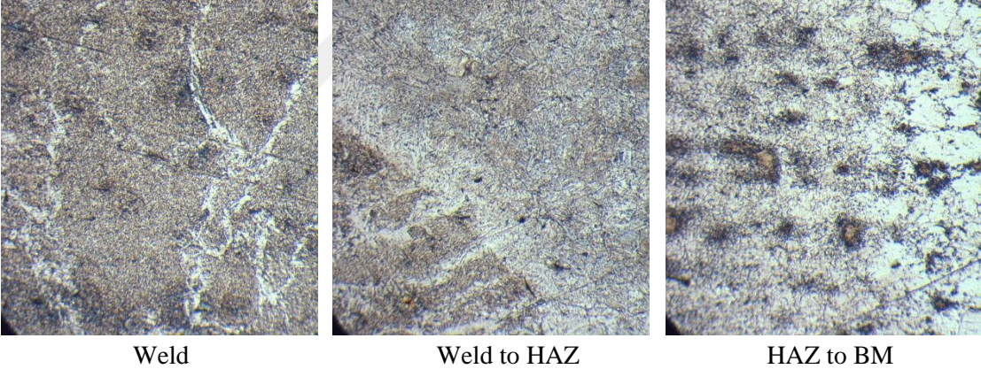
Figure 4.18 The microstructure of four-pass weldment in different zones
