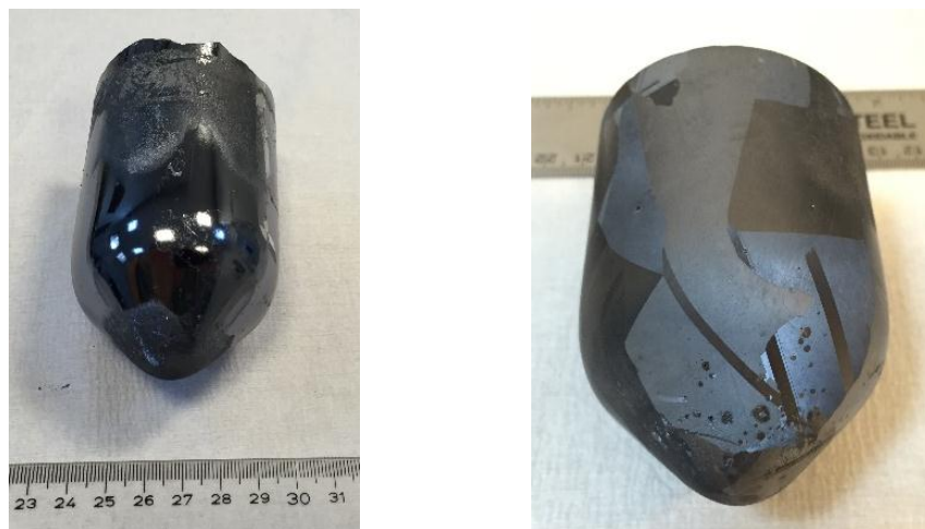
Figure 3.3 MT7 ingot before and after grain revealing etching
