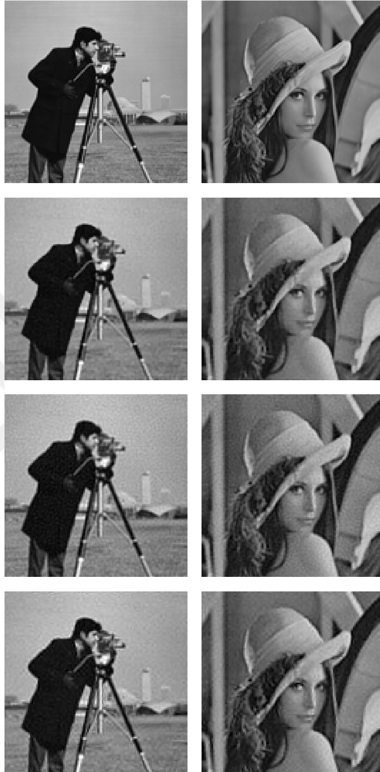
Figure 4.12: From top to bottom: Diffraction-limited NI image pair, reconstructions with DDO, DCT and DWT operators for regularization.
