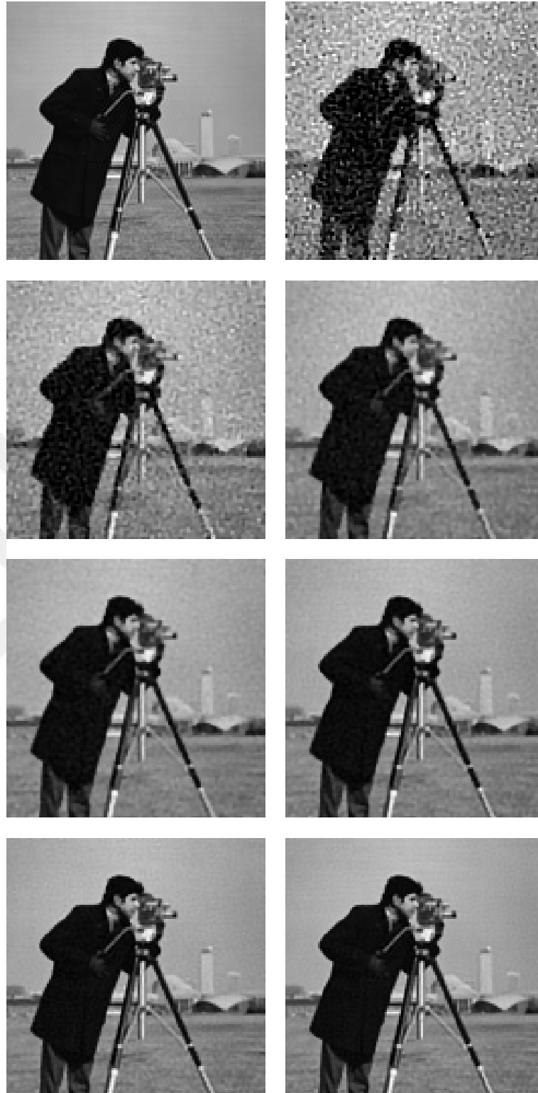
Figure 4.16: Top left: First diffraction-limited intensity image of NI pair. Rest from left to right and top to bottom: Reconstructed images for a measurement noise with SNR values of 10, 15, 20, 25, 30, 35 and 40 dB.
