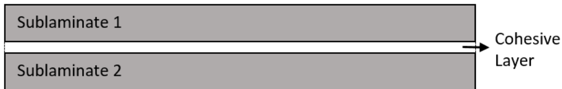
Figure 13: Implementation of cohesive layer
