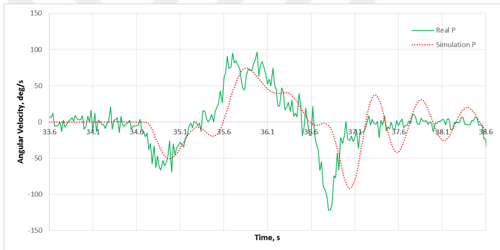
Figure 5.25. The roll rate (deg/s) response to roll stick input in directional motion fixed test setup.
