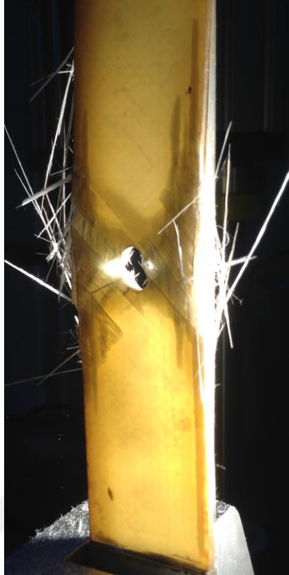
Figure 1-2 Open-hole tension laminate after failure
