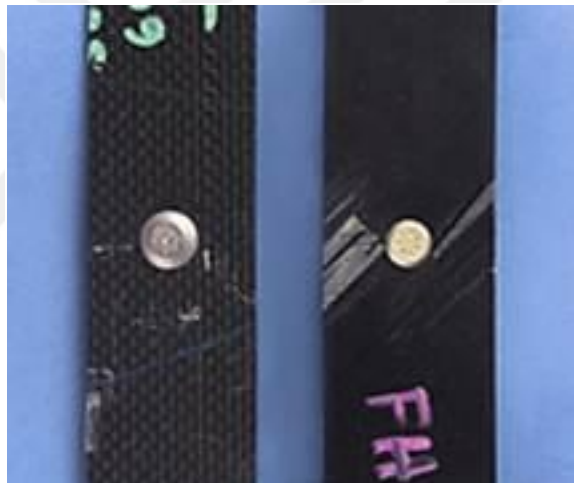
Figure 1-1 Filled-hole tension laminates after failure [7]
