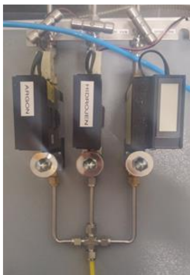
Figure 3. 6: A photo of the digital flow meter
