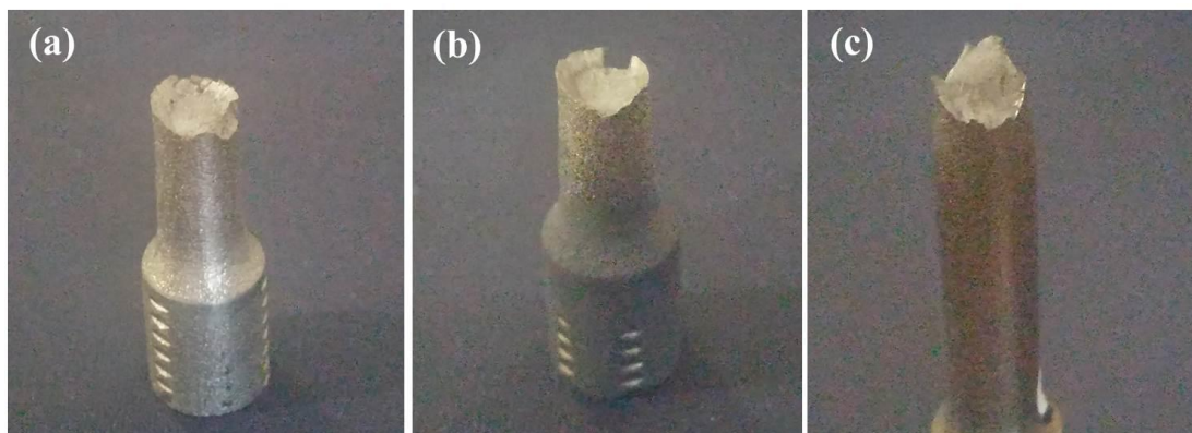
Figure 4. 28: Photos of the macro fracture surface of dumbbell shaped SLM fabricated tensile test; (a) as-received, (b) THP-4 stepped, (c) THP-2 stepped specimens.
