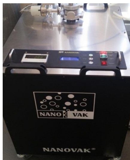
Figure 3. 7: A photo of the vacuum system consisting of rotary and turbo-molecular pump.
