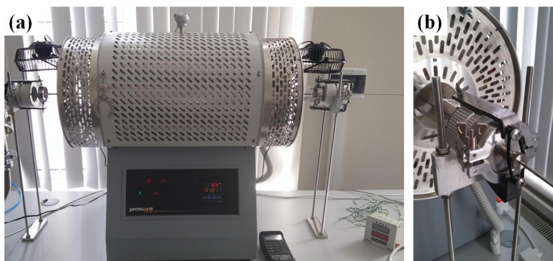
Figure 3. 5: (a) Photos of the heating furnace and the quartz tube; (b) Right hand-end enclosure flange.
