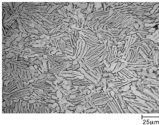
Figure 2. 7: Optical micrograph showing Widmanstätten structure resulted in a casting where \alpha phase in white and \beta phase is dark [19].
