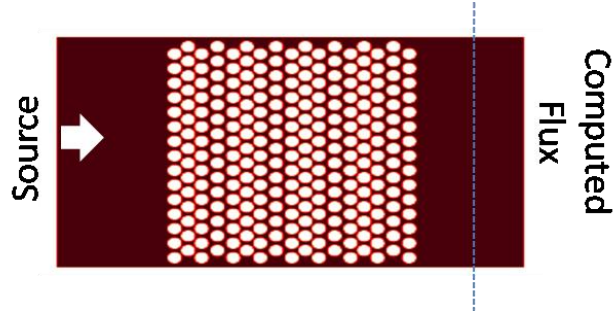
Figure 4.8 - Schematic of Crystal-Crystal superlattice with 3 holes in each side where one column of holes (air) is in common for both sides.
