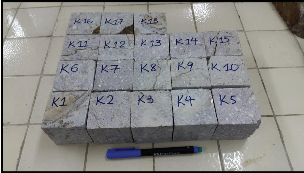
Figure 3.32 Andesite samples used for the laboratory tests.
