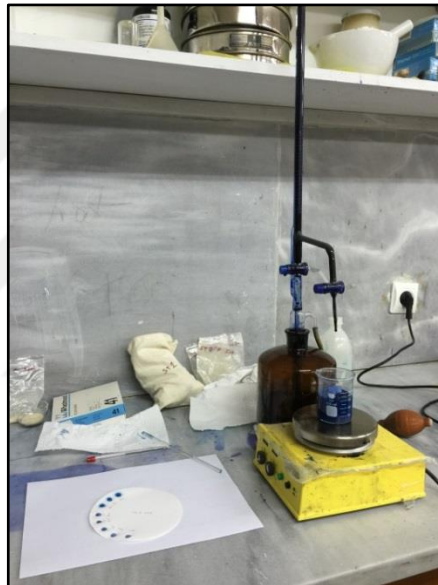
Figure 19. Methylene blue adsorption test equipment used in this thesis
