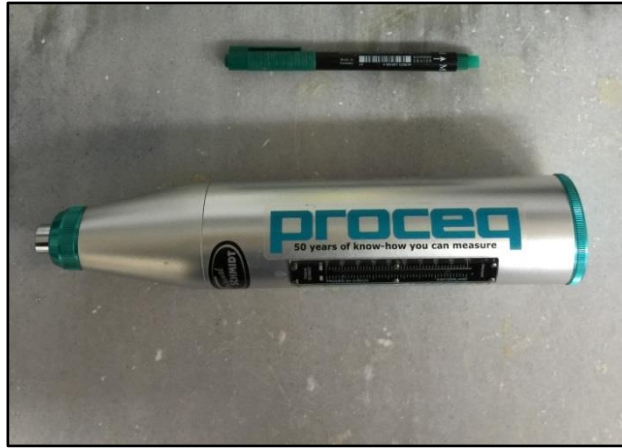
Figure 17. L type Schmidt rebound hammer used in this study
