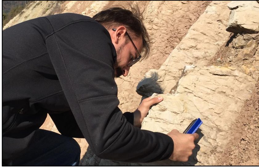
Figure 20. Profilometer used on discontinuity surfaces
