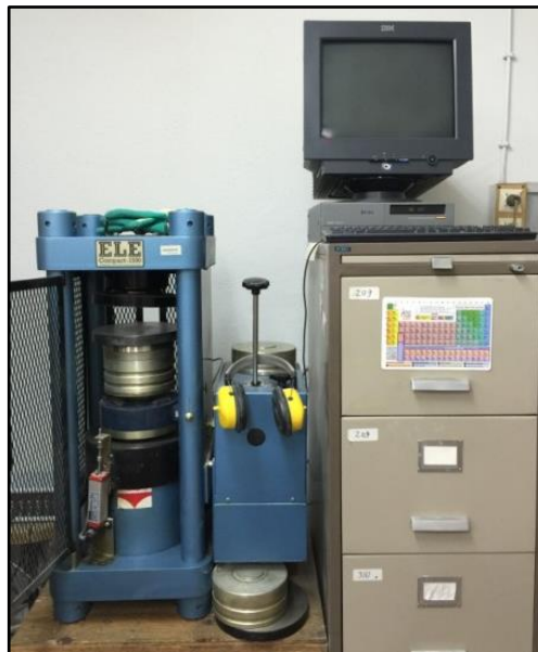
Figure 15. Compression machine used to determine UCS values of the rocks
