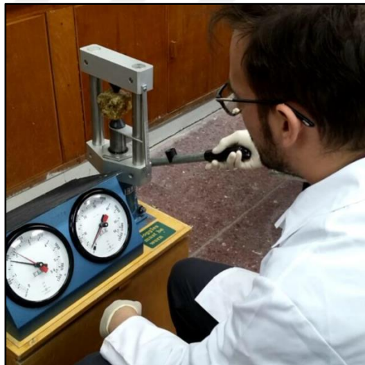
Figure 16. Manual point load device used in this study
