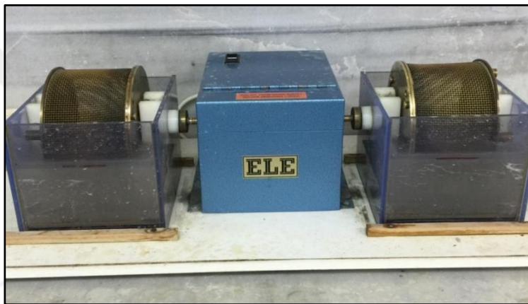
Figure 18. Slake durability test equipment used in this thesis
