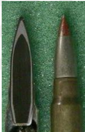
Figure 3 7.62 mm AP Bullet Cut View [21]
