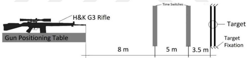
Figure 41 Experimental Test Setup
