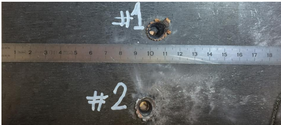
Figure 66 Frontal Image of the Impacted Plate 2-2 Configuration (20 mm Total Thickness)
