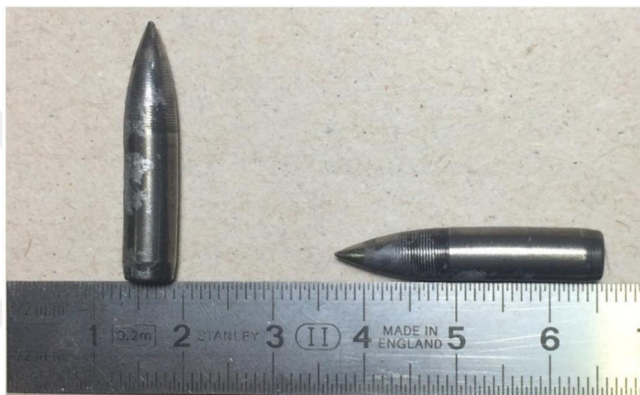
Figure 53 The Bullet Cores Ejected From 27 mm Thick Mild Steel Target
