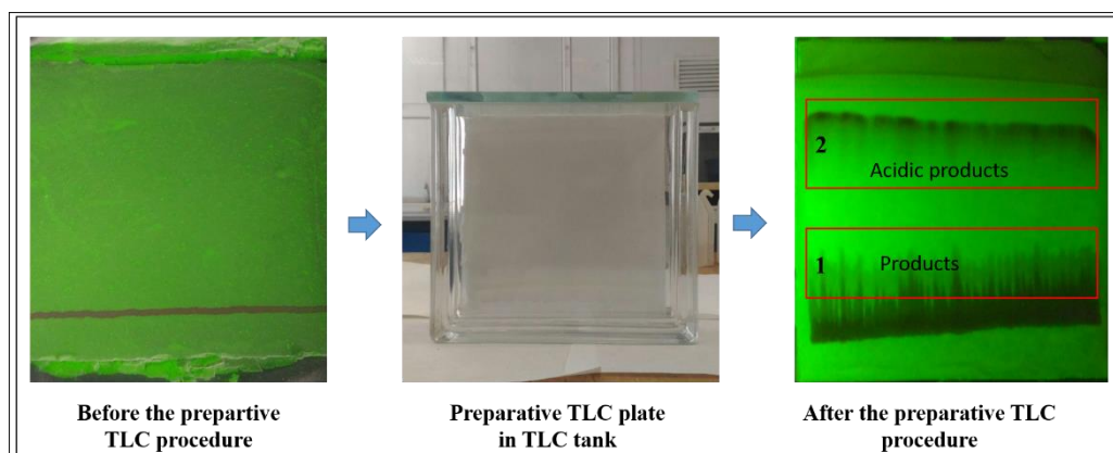
Figure 50 Appearance of preparative TLC plate First plate image shows the thin line of the TPP-DCA prepared by using dichloroacetic anhydride, the last plate shows the separation of the same sample after running with DCM: ethylacetate in 2:1 (v/v)
