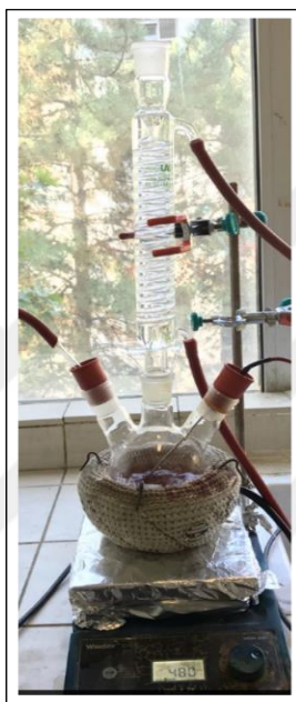
Figure 8. Image of experimental set up of co-precipitation methods
