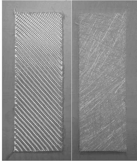
Figure 5.2. Fabric samples, twill (left), mat (right)
