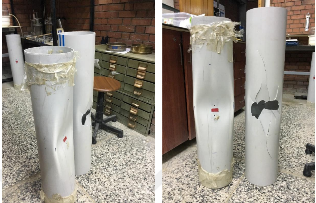
Figure 5.2. Side and front view of the heavily distorted pipe (with red tape) and collapsed pipe
