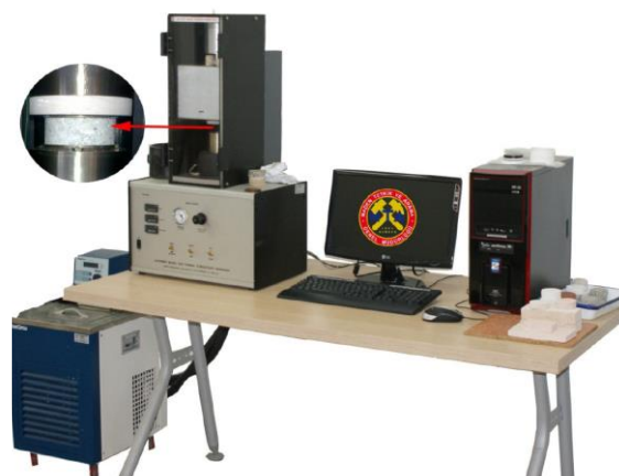
Figure 3.8 Unitherm 2022 thermal conductivity apparatus.
