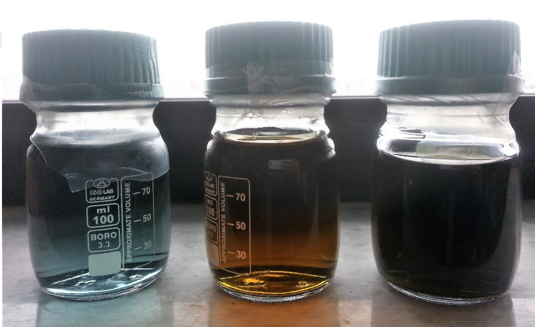
Figure 2.2 Precursor solutions prepared by dissolving \text{MoCl}_5 in UP water. Molarities of the solutions from left to right are 1, 5 and 10 mM respectively.
