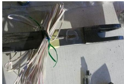
Figure 4-12. Strain gauges installed on a driven bar
