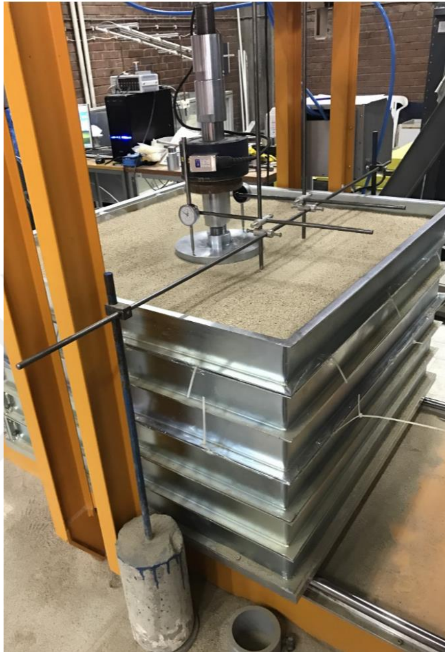
Figure 4.14 Placement of dial gauges by using dial gauge installation system
