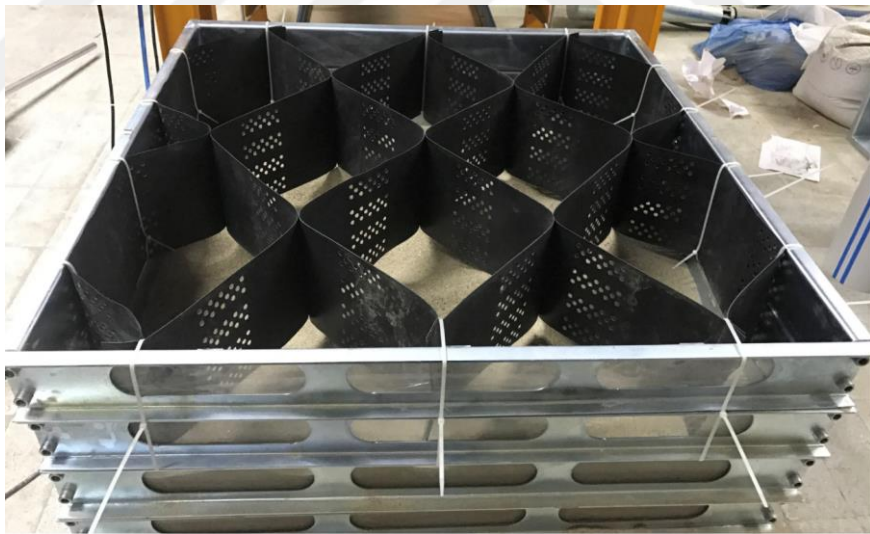
Figure 4.12 Placement of geocell tied segments to sand filled testing tank
