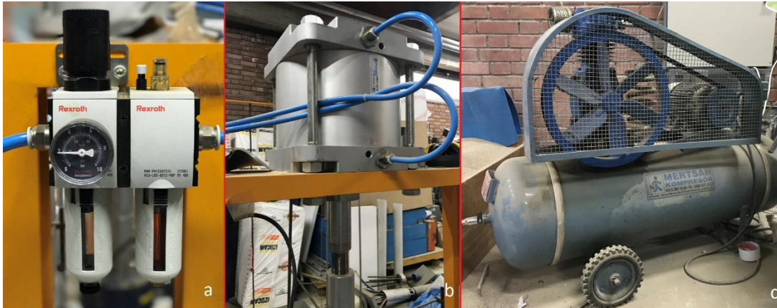
Figure 3.4 Pieces of the loading system (a: pressure regulator valve, b: pneumatic piston, c: air compressor)
