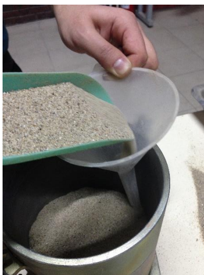
Figure 3.13 Placement of soil using a funnel
