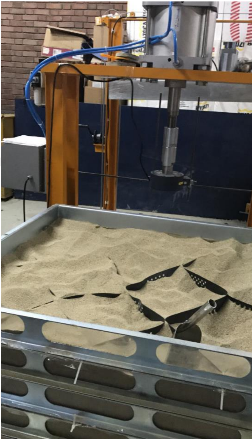
Figure 4.15 Removal of the sand from the tank by a shovel at the end of the test
