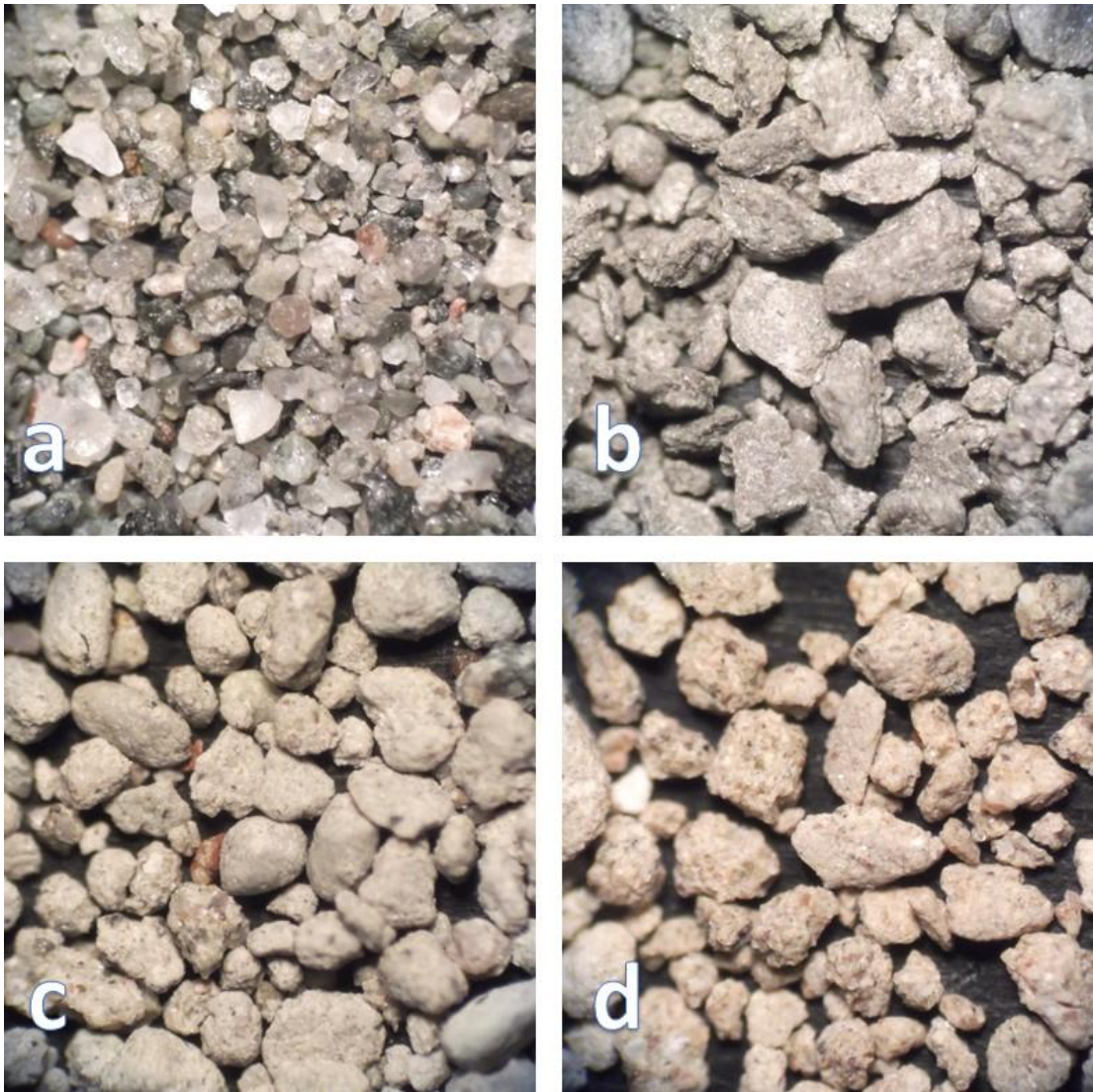
Figure 15: (a) Quartz grains (See EDS analyses APPENDIX A, Figure 25); (a) Black rock fragments (See EDS analyses in APPENDIX A, Figure 26) from GB section, GB-30; (b) Rock grains with calcite matrix (See EDS analyses APPENDIX A, Figure 24) from GÖM section, GÖM-12; (c) Rock grains with calcite matrix from Aksu (IS) section, IS-36 (See EDS analyses APPENDIX A, Figure 22; (d) Rock grains with calcite matrix from Aksu (IS) section, IS-56 (See EDS analyses Appendix A, Figure 23)
