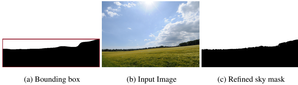
Figure 3.4: Using the input image and the foreground rectangle information as inputs, Grabcut refines the coarse sky mask generated by FCN. Input image taken from [1].
