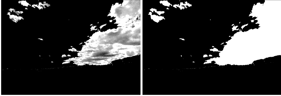
Figure 3.8: Left image is the cloud softness map M_s and the right one is the cloud mask M_c .
