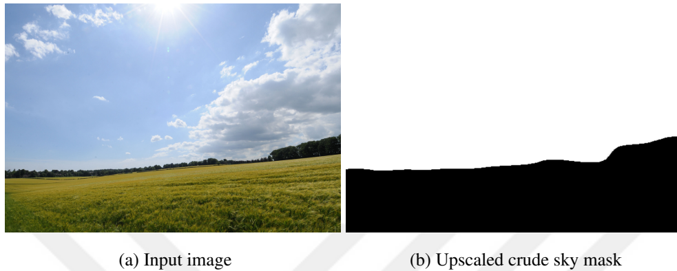
Figure 3.3: Input image and the crude sky mask gathered with the FCN algorithm. Mask is scaled to the size of the input image. Input image taken from [1].
