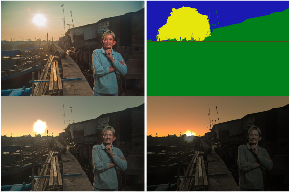
Figure 4.6: Input image, segmentation mask, and relighted outputs after incremental sun movements. Image taken from [11].
