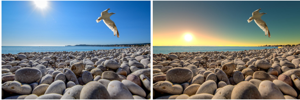
Figure 5.3: After the sun movement the water pixels can not be relighted correctly without the BRDF. Image taken from [9].
