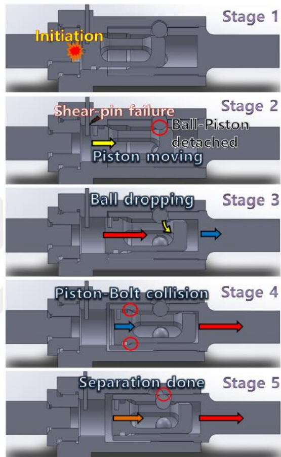
Figure 5: The separation of the ball-type explosive bolts can be realized in five stages. At the first stages, the initiator is electrically ignited and consequently, the gas flows through the piston and shear pin breaks after reaching the critical value at Stage 2. After a while, at Stage 3, the balls between the bolt body and piston drop into the piston and finally, the separation starts with the collision of the piston and bolt body [14].
