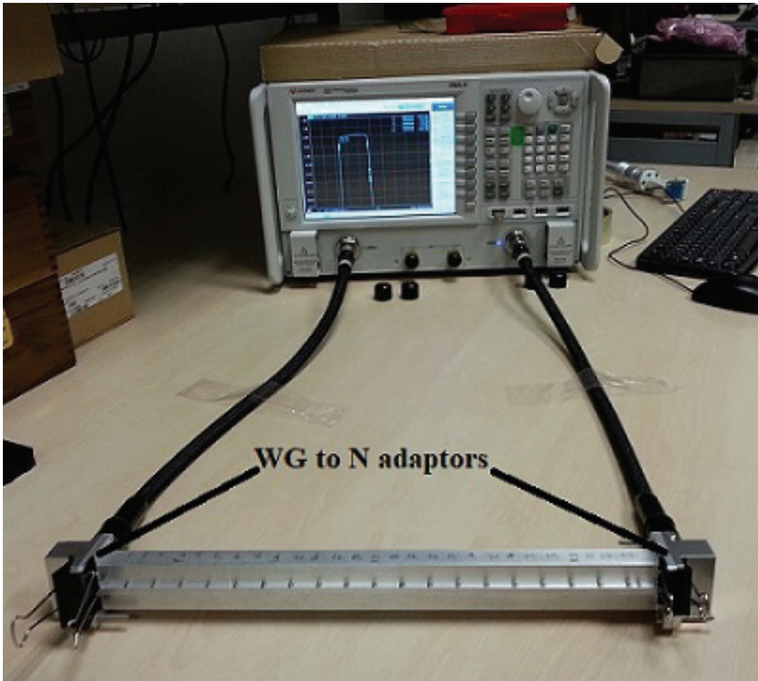
Figure 3.10: 13 th order filter measurement set up
