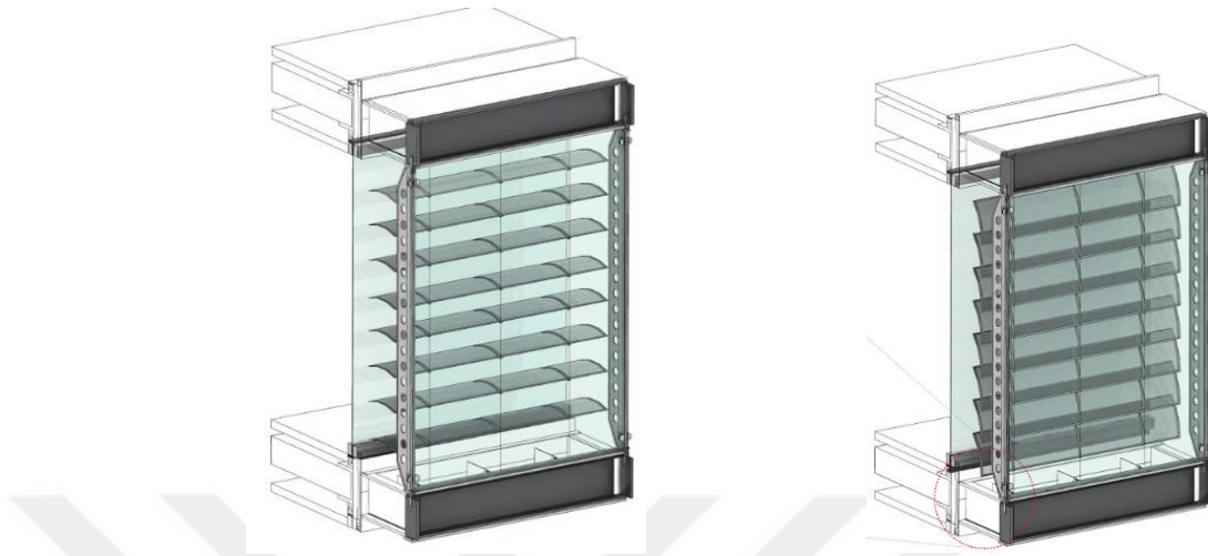
Figure C.63. Double-skin façade with perforated metal louvers. Left: open louvers in early morning hours, right: closed louvers to block direct solar radiation in west façade (Vassigh & Chandler, 2012, p.88).
