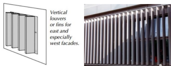
Figure C.20. Vertical shading device (US. Department of Energy).
