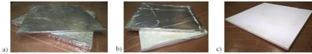
Figure C.4. VIP Samples: (a) VIP 10 and 30 mm thick; (b) punctured VIP and VIP core material; (c) Extruded polystyrene (XPS) (Lorenzati, et al., 2017).
