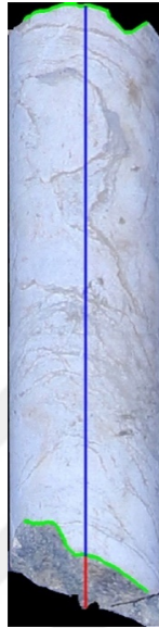
Figure 53. Detected centerline of a core
