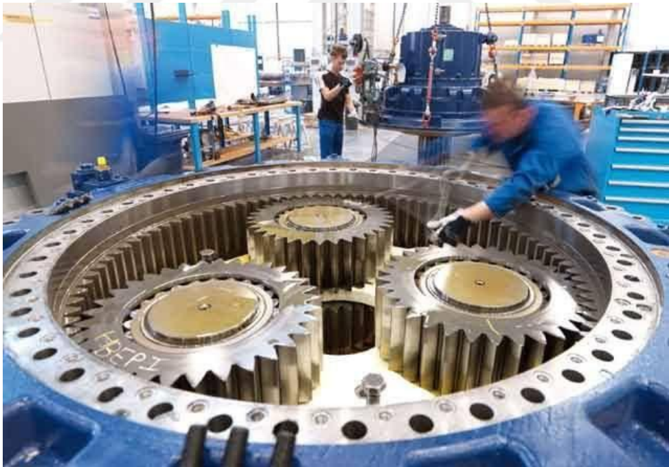
Figure 1-3 Planetary gearbox for a wind turbine [5]
