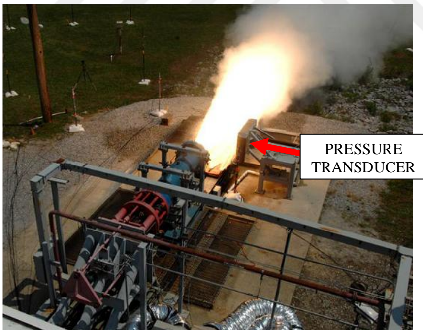
Figure 44: Example of the Pressure Level Measurement by Using Second Type of Pressure Transducer [57]
