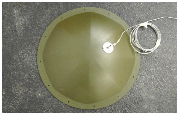
Figure 41: Pressure Transducer Integrated Cover
