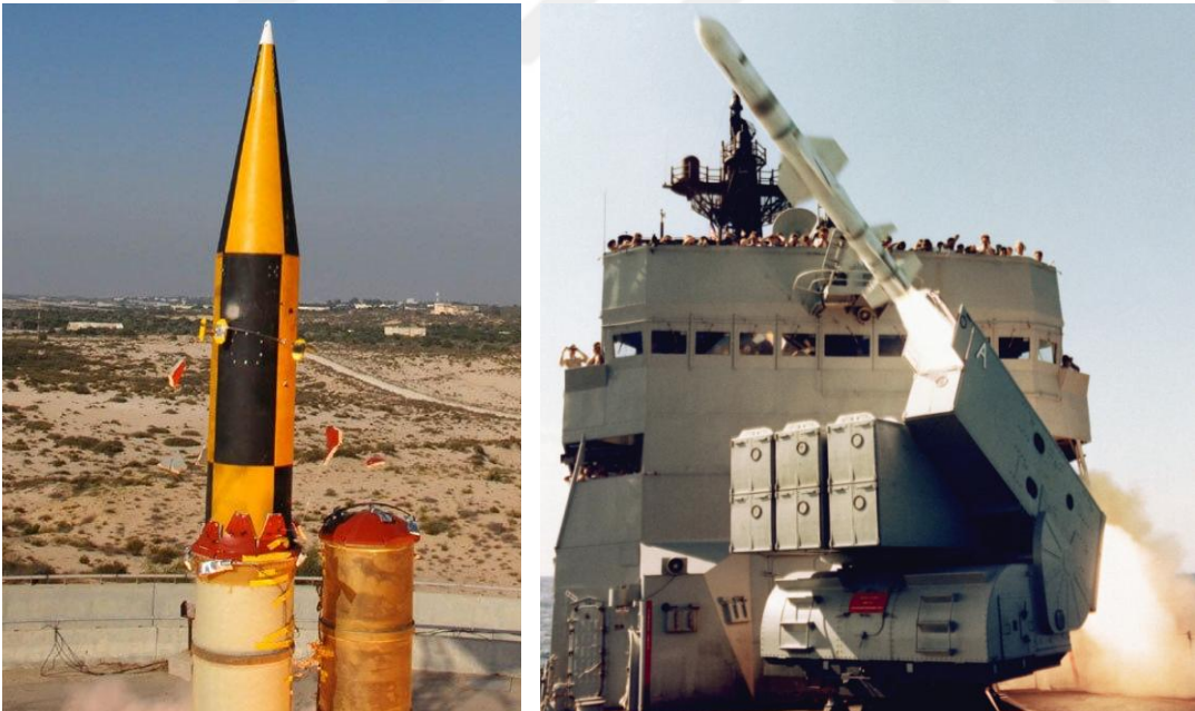
Figure 1: Test Launch of Arrow 3 Missile (Left) [1], RGM-84 Harpoon SSM was Launched from an Mk-16 (Right) [2]
