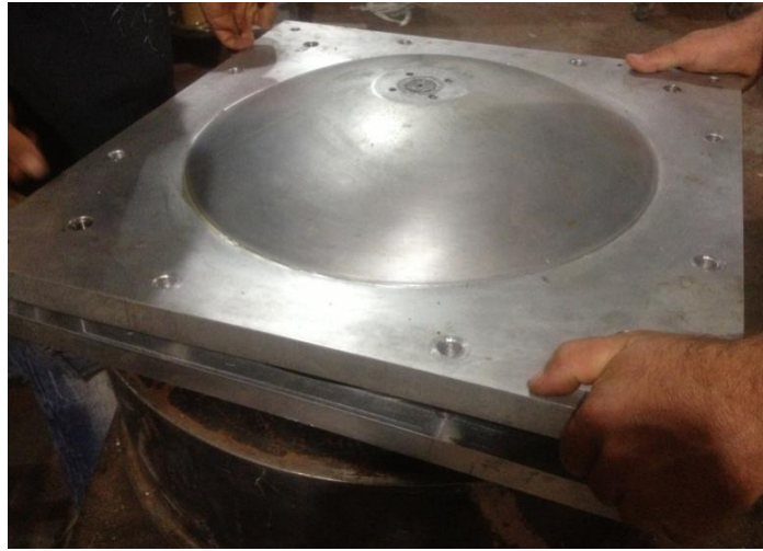
Figure 118: Closing Mold Sections
