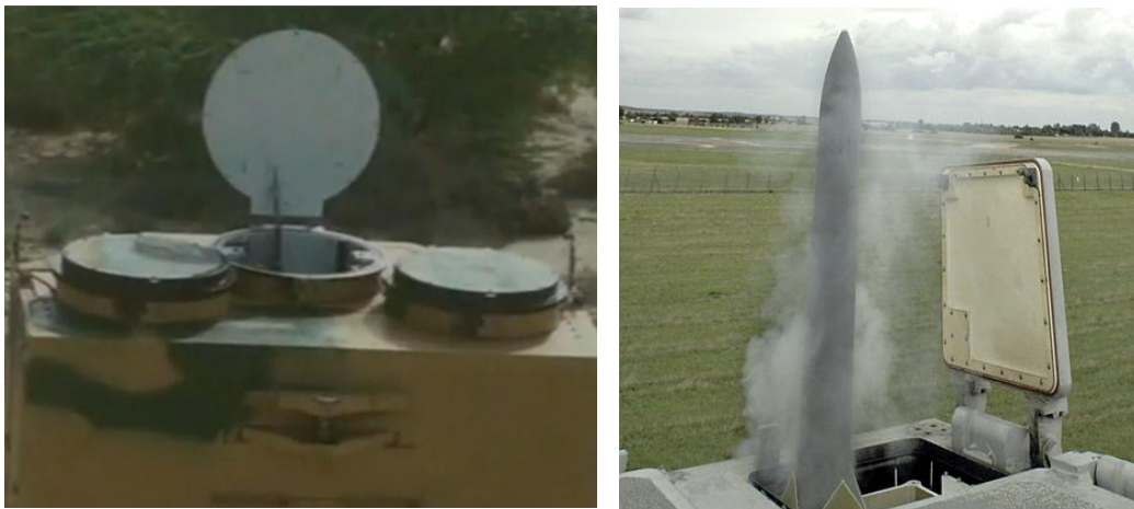
Figure 6: Photographs of Hatch Cover Systems of Babur Missile [12] (Left) and Common Anti-air Modular Missile (CAMM) launching from Lockheed Martin's MK 41 Vertical Launching System (VLS) [13] (Right)
