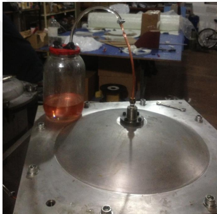
Figure 119: Outlet of Excess Resin
