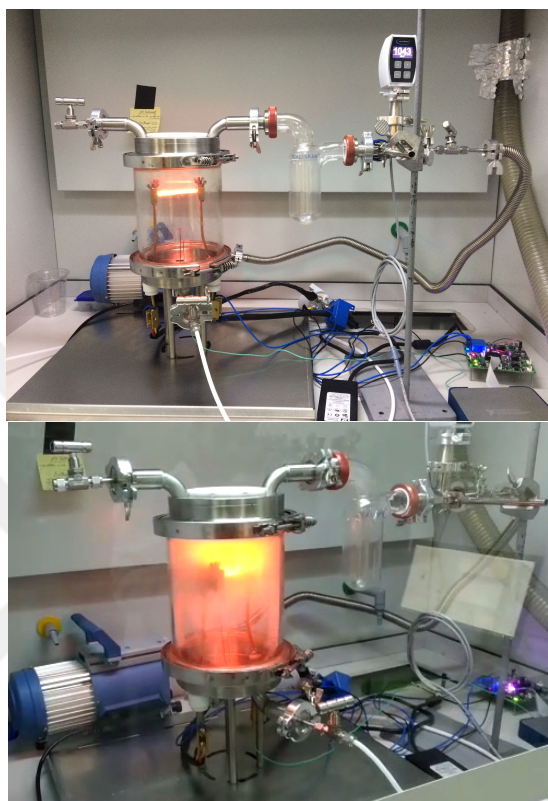
Figure 3.21 Pyrolysis at 4500 °C/s by using molybdenum wire mesh. In the first image, no sample was placed. In the second image, hazelnut shell (HS) was pyrolyzed at 1550 °C.
