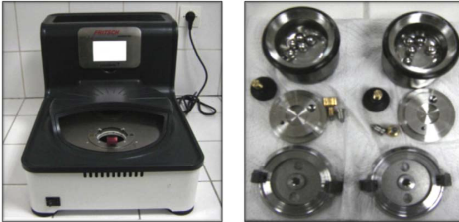
Figure 3.4: The Fritsch Planetary Micro Mill Pulverisette 7, stainless steel bowl and balls
