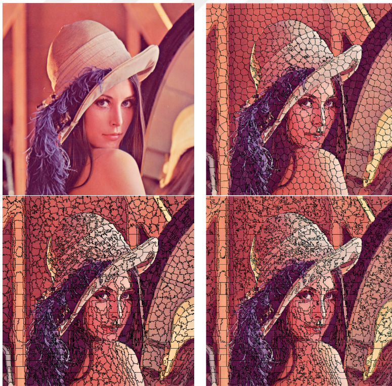
Figure 3.1: RGB image and SLIC superpixels on RGB image for different m values
