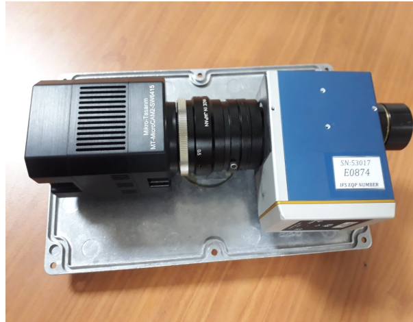
Figure 5.4: SWIR camera and LCTF
