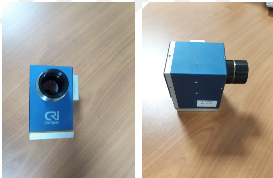
Figure 5.3: Liquid Crystal Tunable Filter (LCTF)
