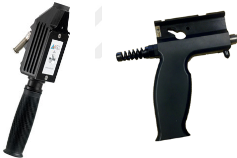
Figure 5.6: a) Contact probe of ASD spectroradiometer b) pistol grip of ASD spectroradiometer
