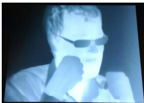
Figure 2.2. A thermal image formed using a photon detector, cooled by a Joule-Thomson cooler
