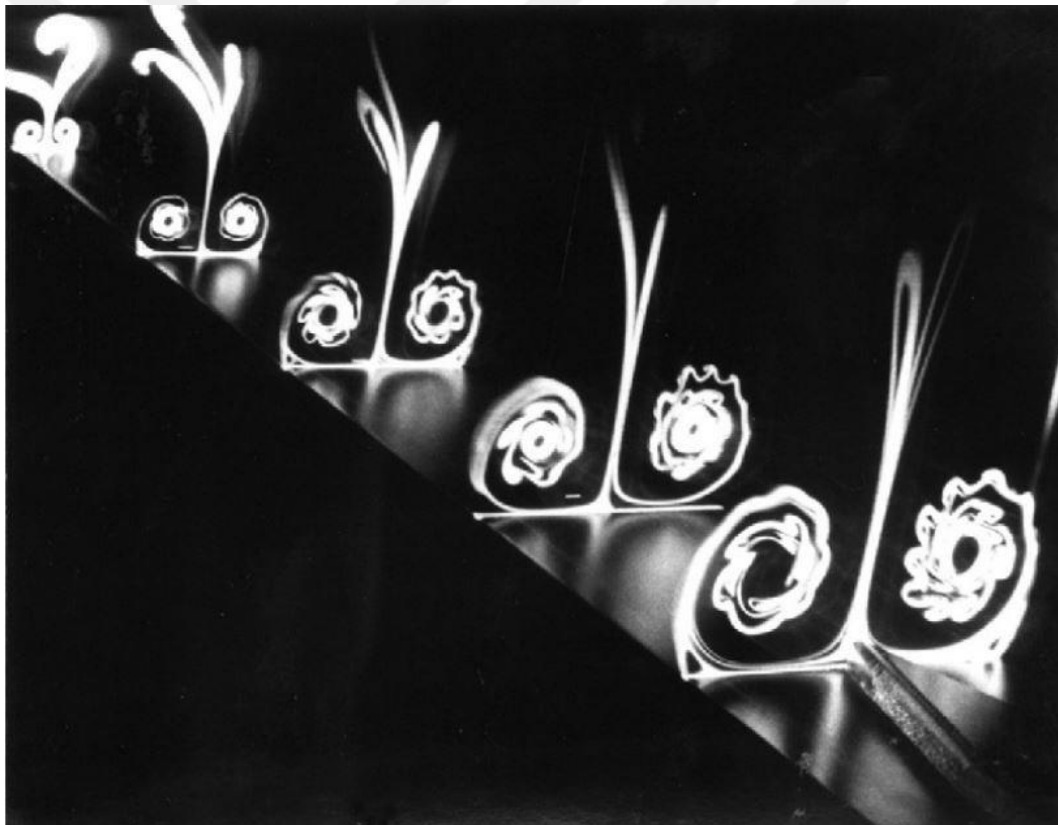
Figure 2.2 Laser light sheet illumination of primary vortices and the discrete vortices that are feeding them [17].
