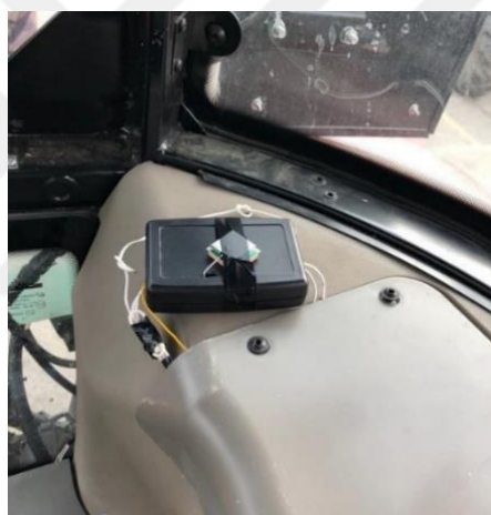
Figure 4.7. Data acquisition and storage unit
